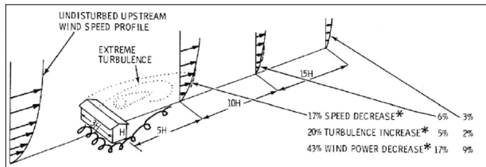
**Figure 6: turbulence effect due to building (Jackson, 2009)**
