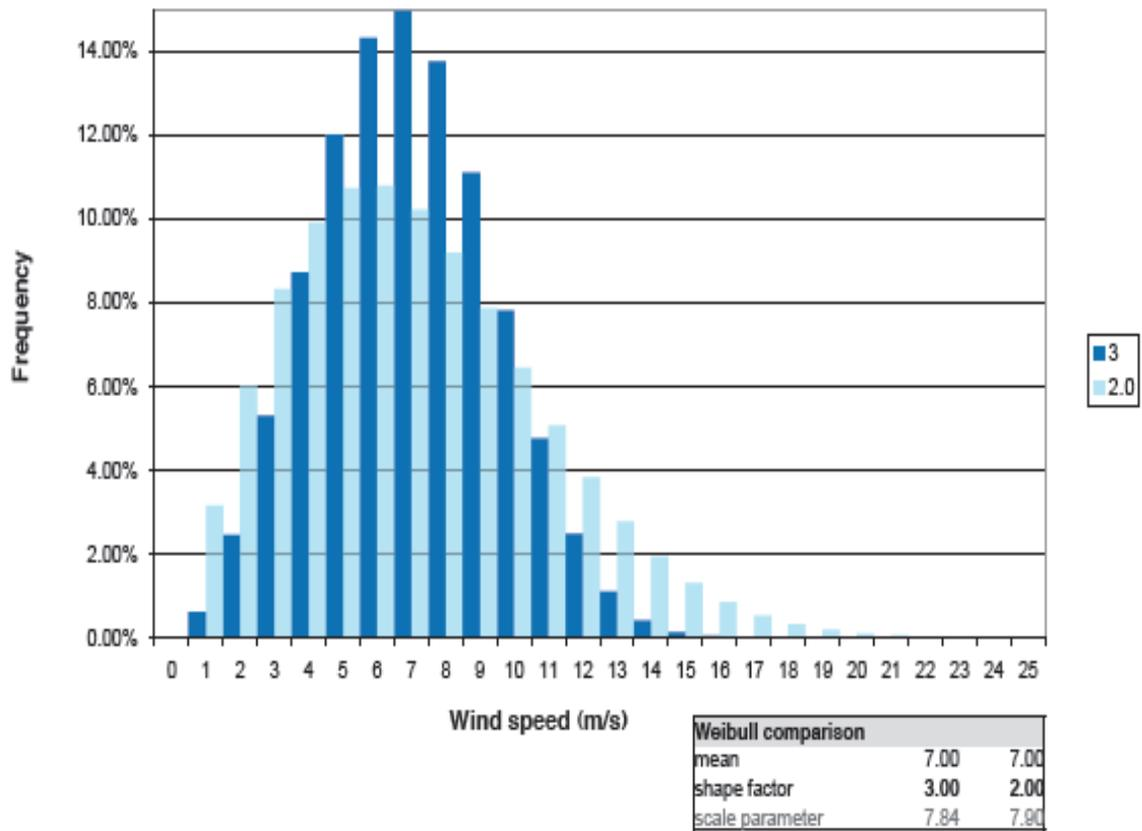
**Figure 4: Two Weibull curves with different shape factors but same mean wind speed. (Jackson, 2009)**
