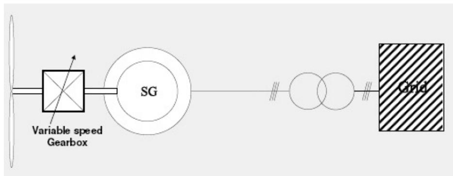
**Figure 14: a typical wind turbine: propeller, gearbox, synchronous generator, transformer connected to the grid (Jackson, 2009)**
