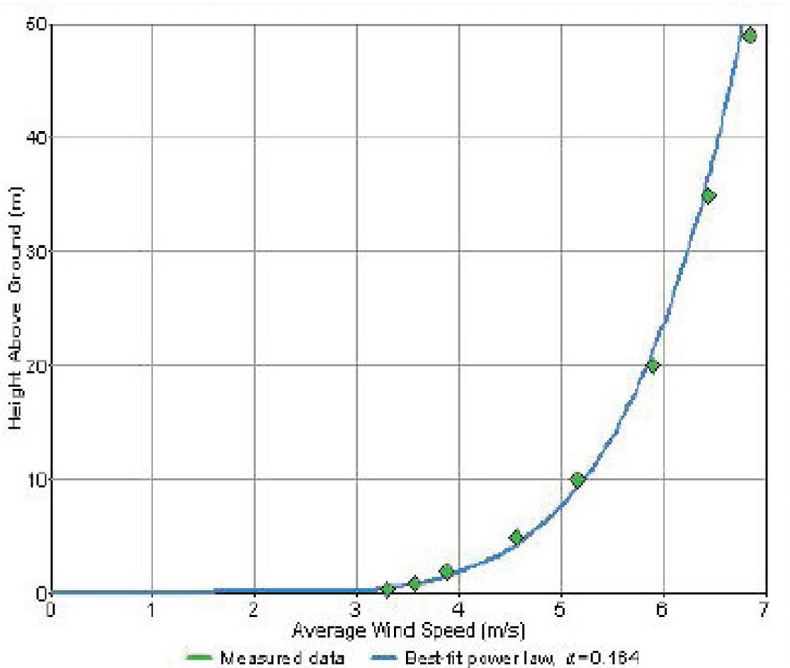
**Figure 7: wind shear profile (Jackson, 2009)**
