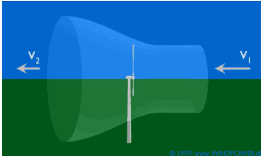
**Figure 57: a wind turbine in a Betz tube**
