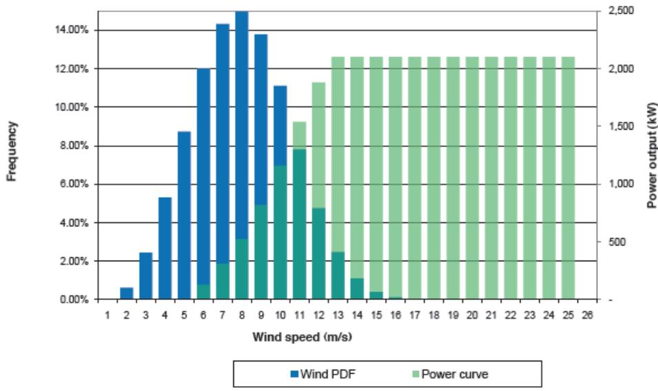
**Figure 10: wind speed distribution vs. power curve (Jackson, 2009)**
