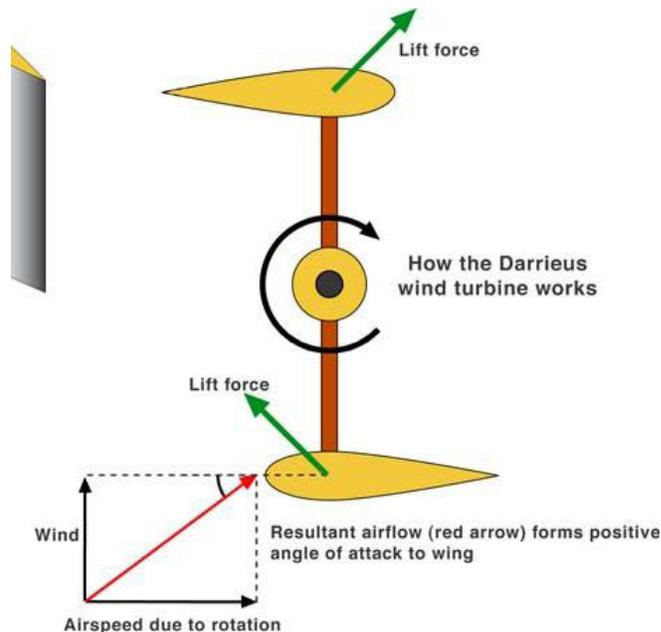
**Figure 15: how the Darrieus turbine works (Jackson, 2009)**
