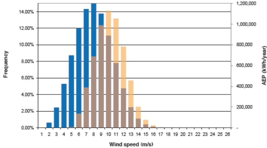
**Figure 11: wind speed, power and AEP (Jackson, 2009)**
