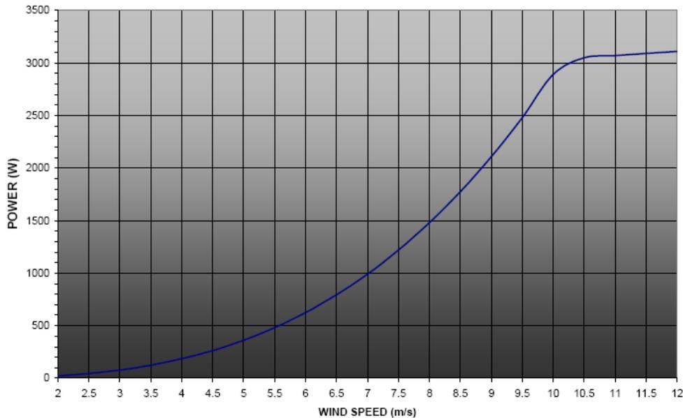
**Figure 3: Example of a power curve (Kestrel Wind)**
