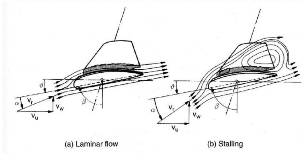
**Figure 5: Laminar flow and stalling due to turbulence (Jackson, 2009)**
