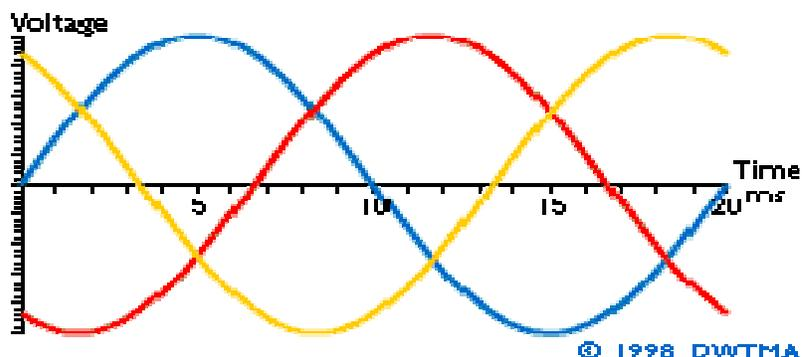
**Figure 13: Three phase electricity (DWTMA)**
