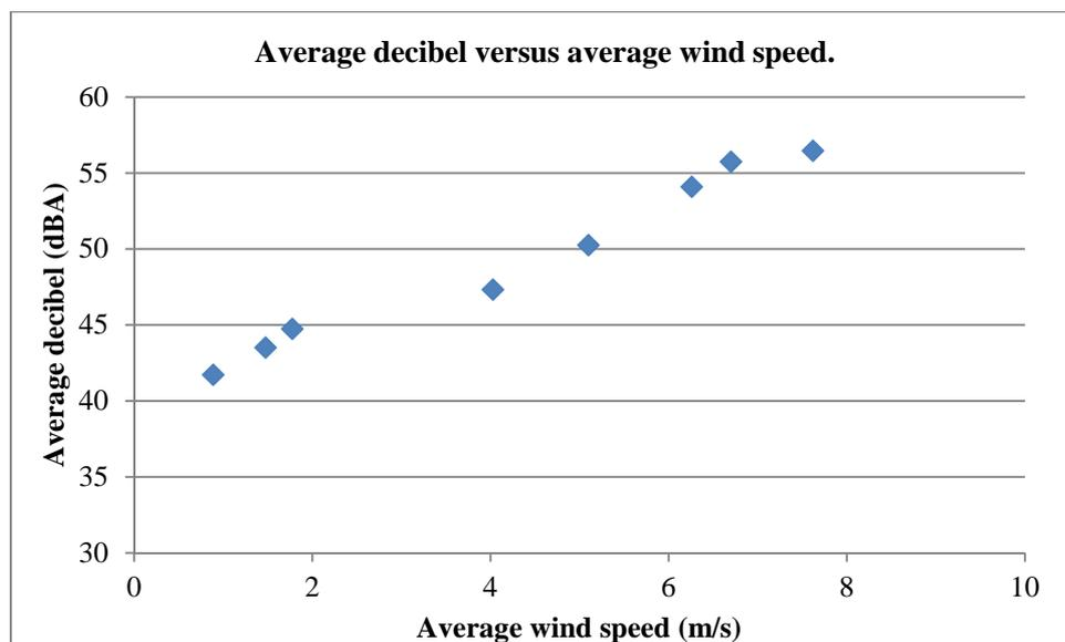
Figure 5.7: Affects of Wind Speed on Average SPL for the vertical axis micro-wind turbine.
