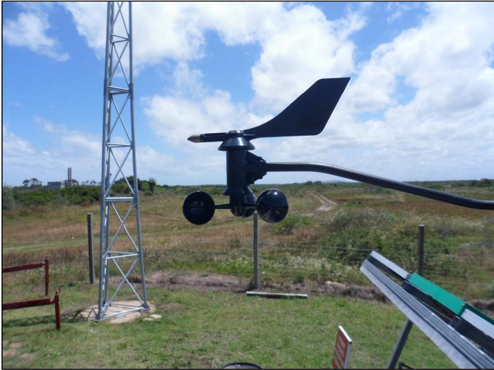
Figure 3.1: WSD-100 Wind Speed and Direction Sensor.
