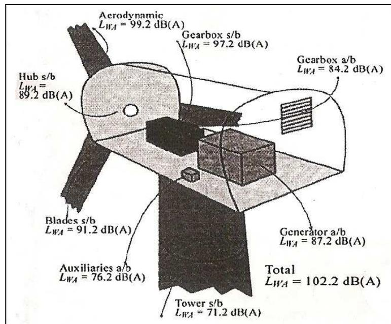
Figure 2.11: Components and total Sound Power Levels of a 2 MW wind turbine, showing the structure-borne and air-borne transmission paths (Rogers et al, 2006).
