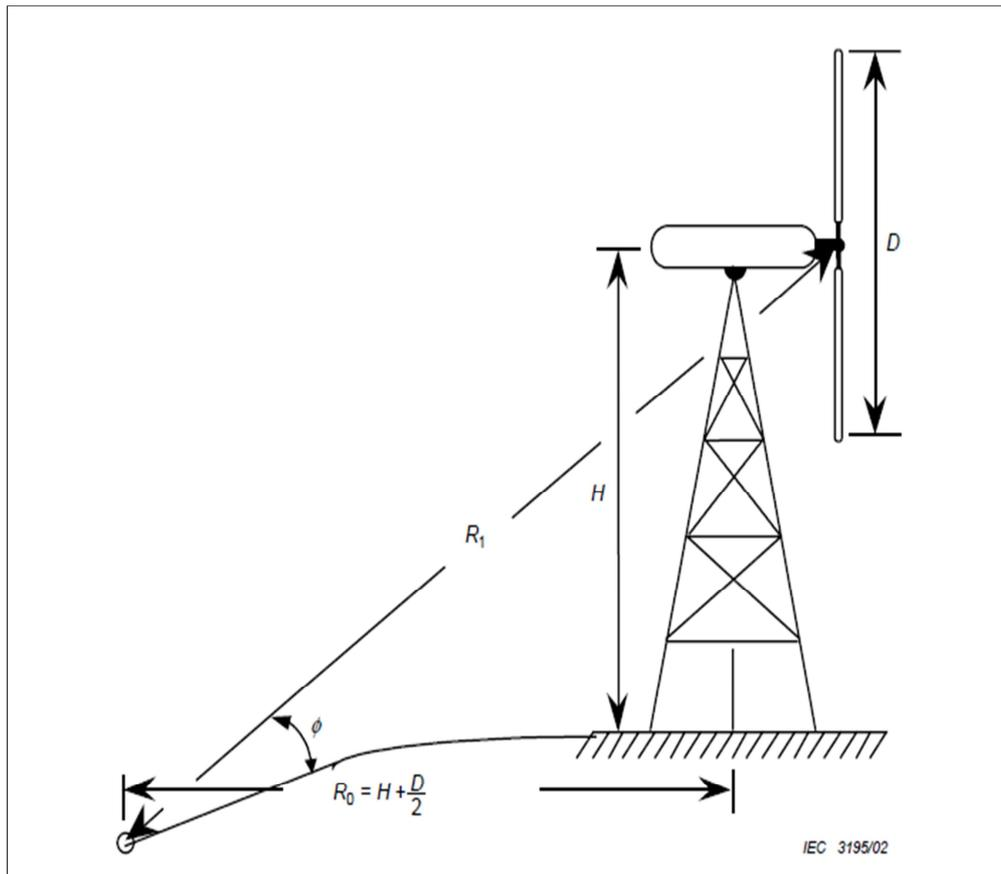
Figure 3.4: Reference position  $R_0$  (IEC 61400-11.2002).
