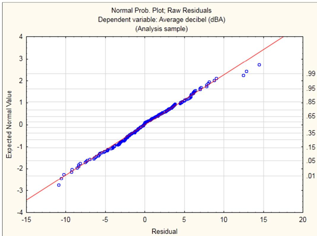
Figure B.2: Normal probability plot of the residuals of reduced model one including interaction.
