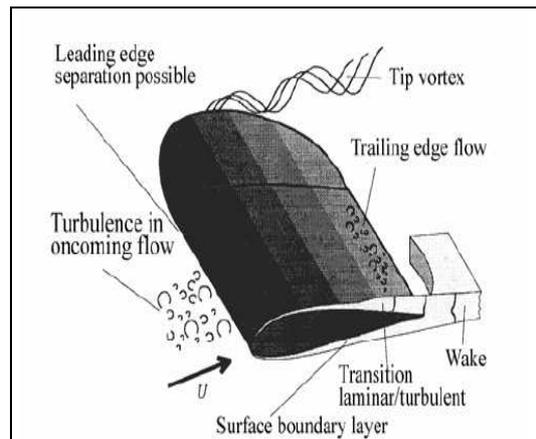
Figure 2.10: Air flow across the blade section (Brown, 2010).
