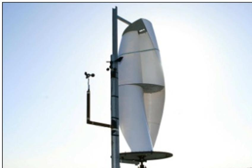
Figure 2.2: Vertical axis micro-wind turbine.
