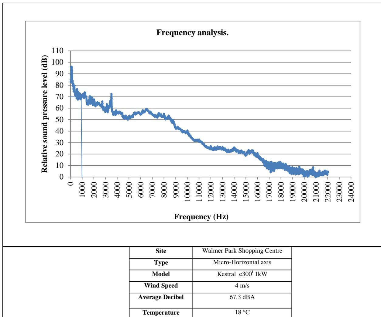
Figure 5.6: Frequency distribution of a sound recording of the horizontal axis micro-wind turbine
