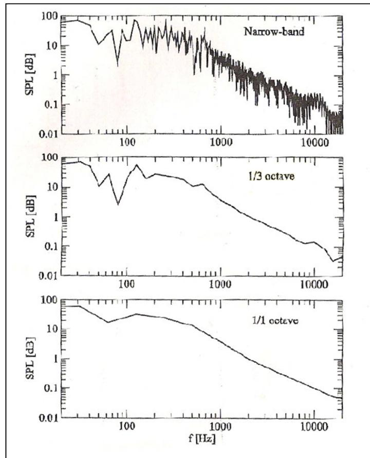
Figure 2.6: Narrowband, 1/3 octave band and 1/1 octave band of the same acoustic pressure signal (Szasz and Fuchs, 2008).
