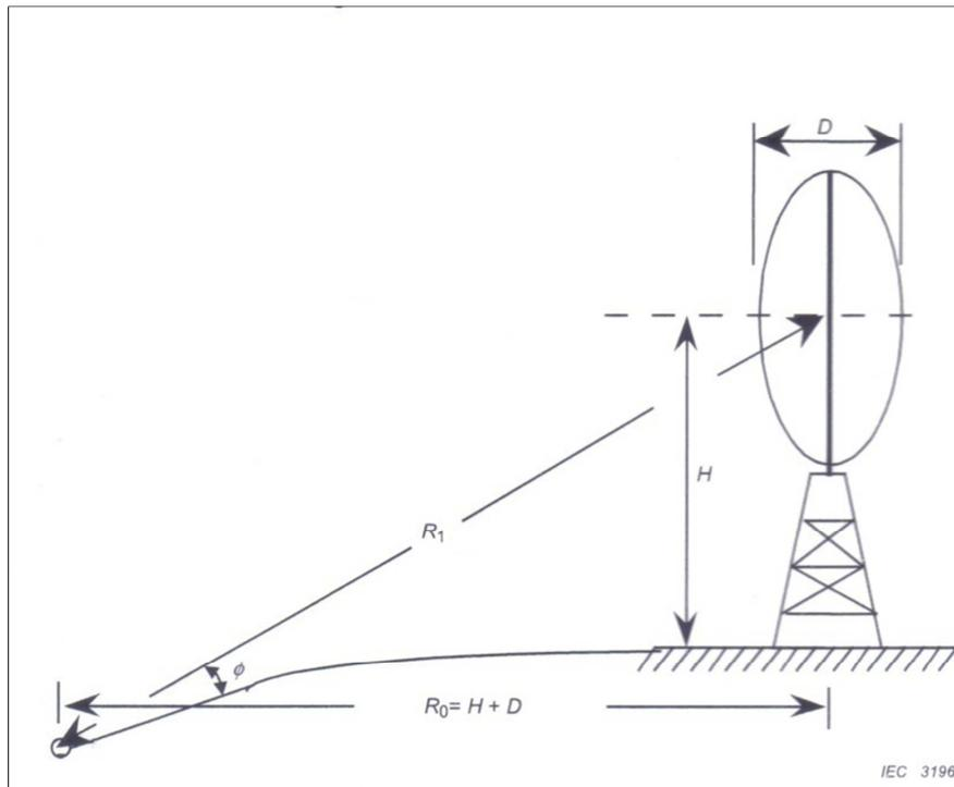
Figure 3.5: Reference position  $R_0$  (IEC 61400-11.2002).
