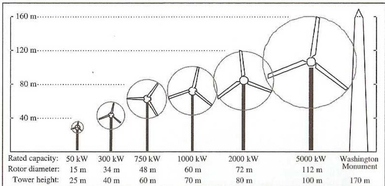
Figure 2.1: Representative size, height, and diameter of wind turbines (Manwell et al, 2007).
