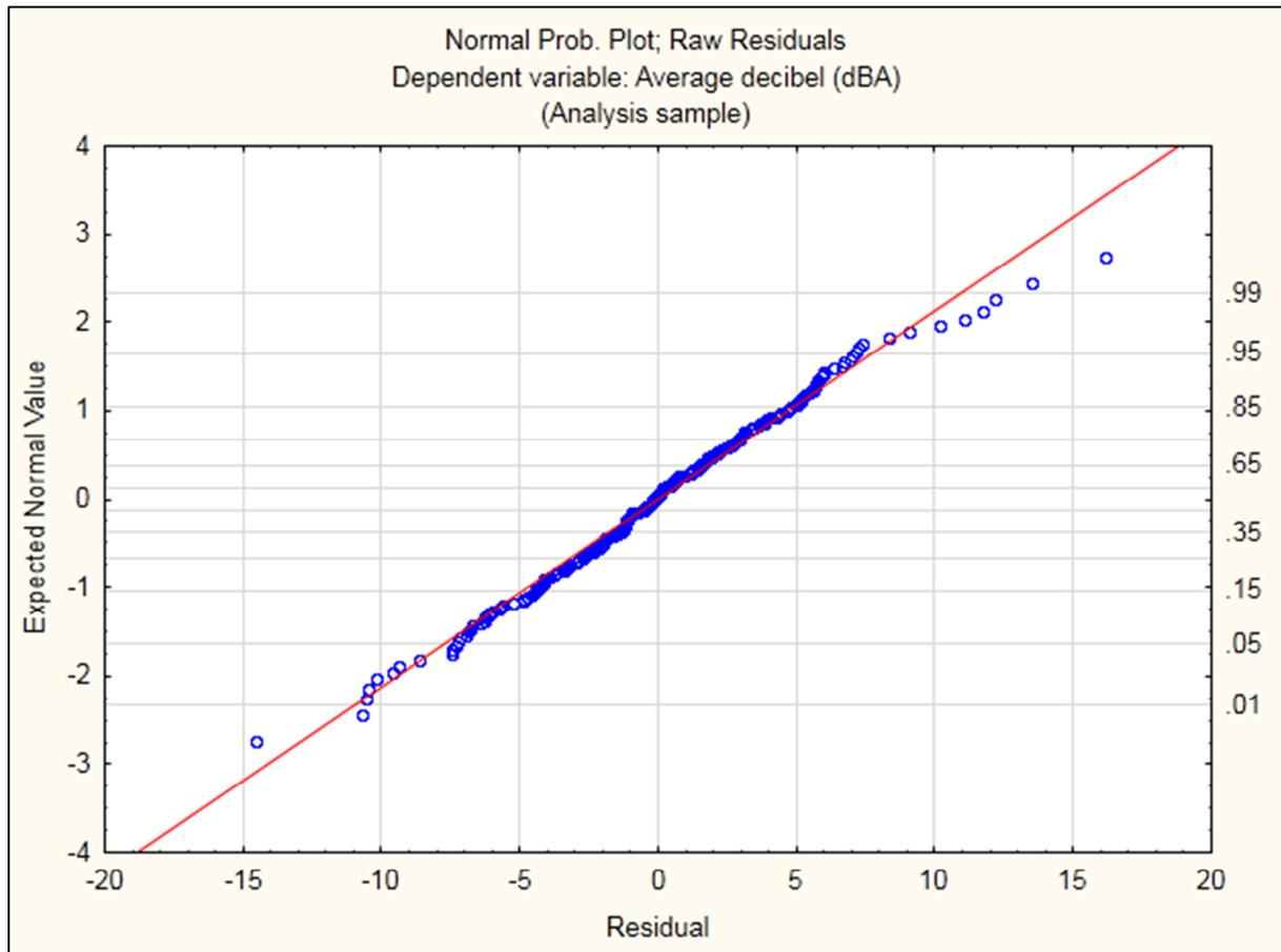
Figure B.1: Normal probability plot of the residuals of reduced model one.
