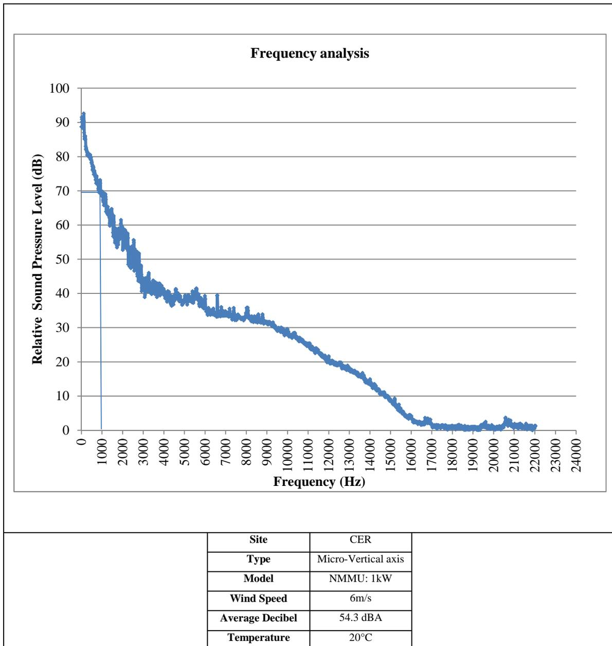
Figure 5.9: Frequency distribution of a sound recording of the vertical axis micro-wind turbine.
