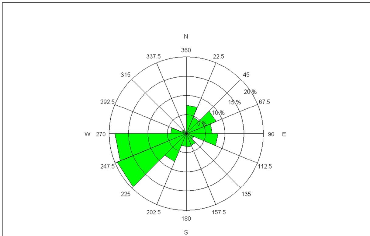
Figure 5.2: Wind rose plot for the Summerstrand, PE region for wind direction data from January 2011 to October 2011.
