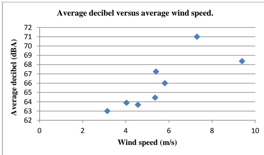
Figure 5.3: A plot of wind speed versus the average SPL reading for the horizontal axis micro-wind turbine.
