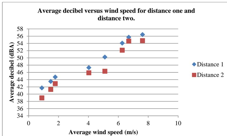
Figure 5.8: A plot of wind speed versus the average SPL for the horizontal axis micro-wind turbine for two different distances.
