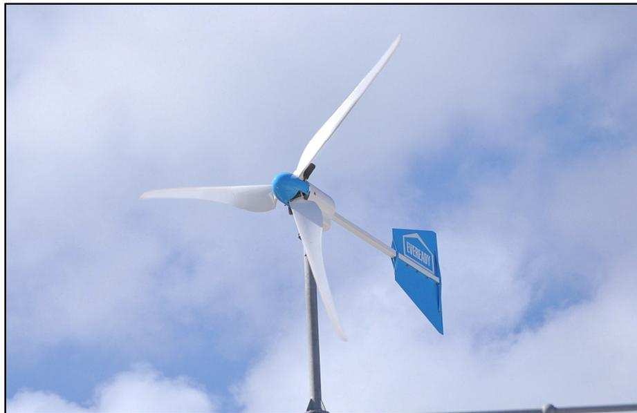
Figure 2.3: Horizontal axis micro-wind turbine.
