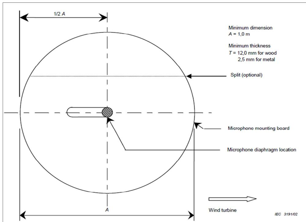
Figure 3.3: Mounting of the microphone-plan view (IEC 61400-11.2002).
