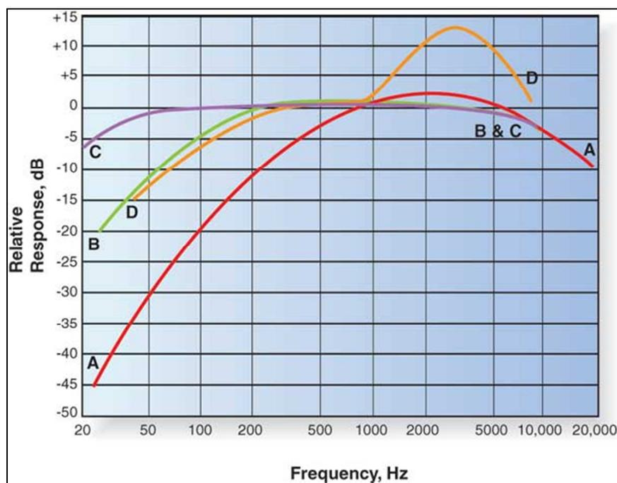
Figure 2.8: Acoustic Weighting Curve (Retrieved on the 13<sup>th</sup> of November 2011 from [www.extron.com](http://www.extron.com)).
