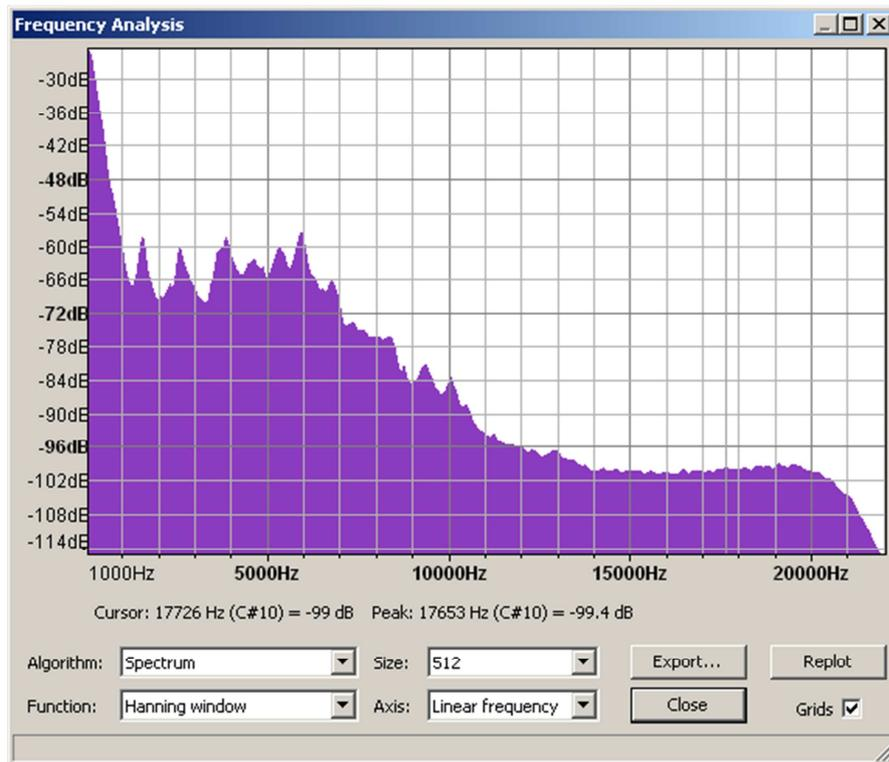
Figure 3.6: Example of the Power Spectrum in Audacity.
