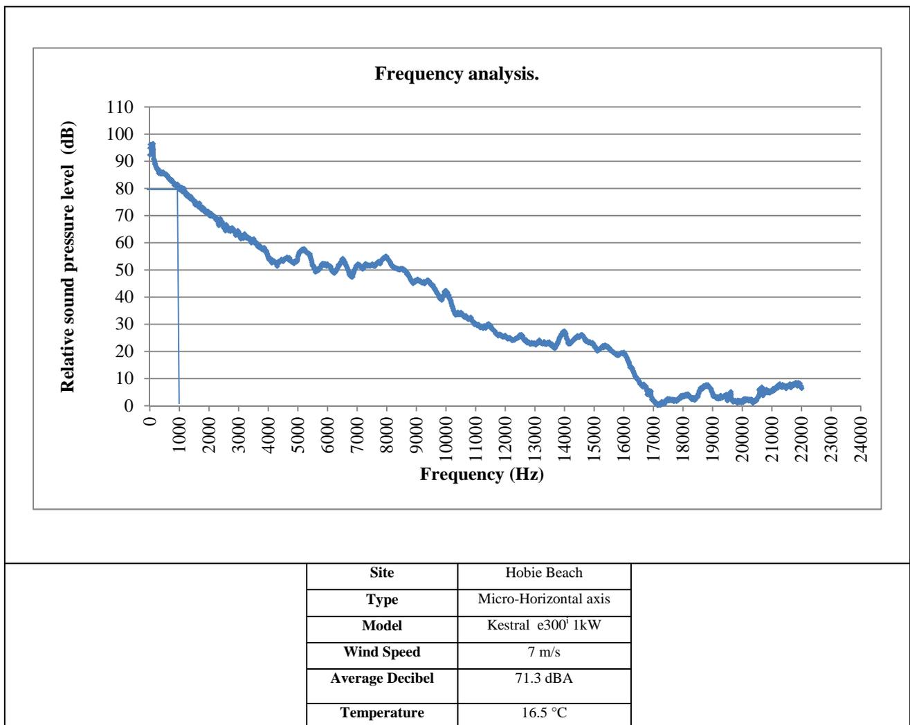
Figure 5.5: Frequency distribution of a sound recording of the horizontal axis micro-wind turbine.
