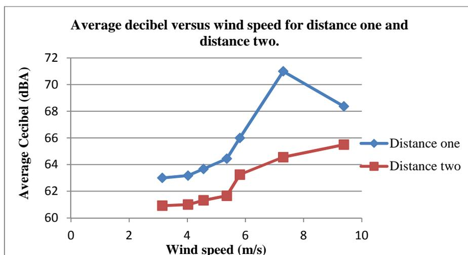
Figure 5.4: A plot of wind speed versus the average SPL for the horizontal axis micro-wind turbine for two different distances.
