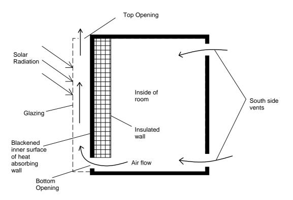
Figure 1.1: Solar chimney as part of the exterior wall of a building
