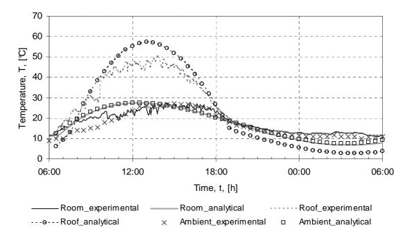
Figure 6.2: Comparison of experimental and analytical data for summer operation
