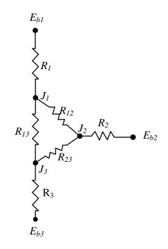
Figure C.3: Resistance network for radiation model
