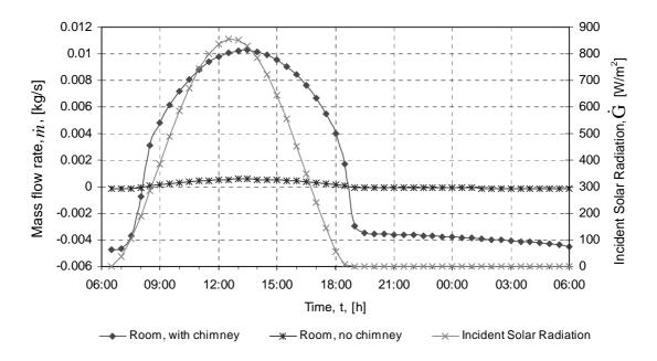
Figure 5.13: Mass flow rates for summer operation
