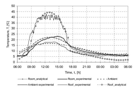
Figure 6.1: Comparison of experimental and analytical data for winter operation
