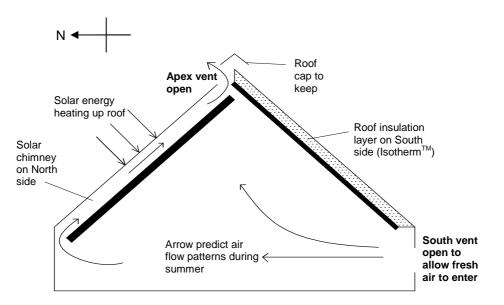
Figure 4.4: Expected operation of test-rig during summer
