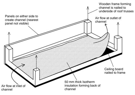
Figure 4.2: Construction of the solar chimney's lower section
