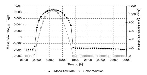
Figure 5.10: Mass flow rate and incident solar radiation for winter operation
