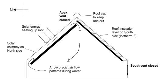
Figure 4.5: Expected operation of test-rig during winter
