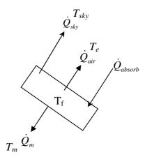
Figure 5.2: Control volume for roof section
