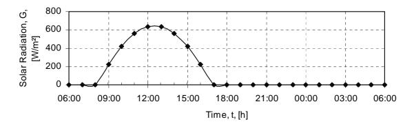
Figure B.1: Incident solar radiation on a horizontal plate in winter (sunny day)
