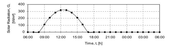
Figure B.2: Incident solar radiation on a horizontal plate in winter (cloudy day)
