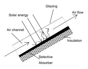
Figure 2.1: Sketch of conventional chimney design
