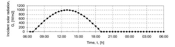
Figure B.7: Incident solar radiation on a horizontal plate for summer
