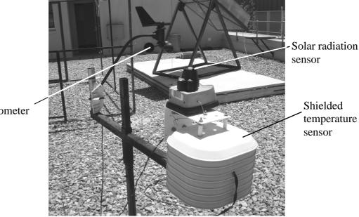
Figure 4.7: Weather station set up near test-rig
