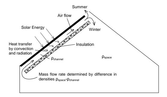
Figure 2.3: Principle of roof solar chimney concept
