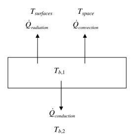
Figure C.5: Wall inner boundary control volume
