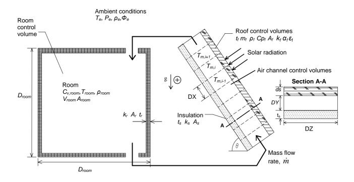
Figure 5.1: Most important parameters of winter analytical model
