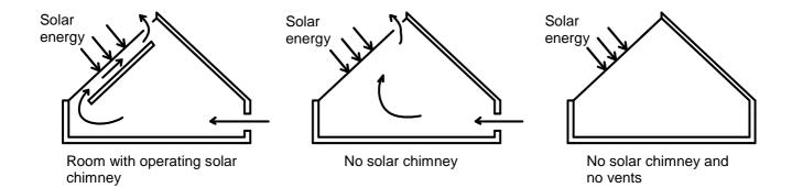
Figure 5.11: Three simulation models for summer operation comparison
