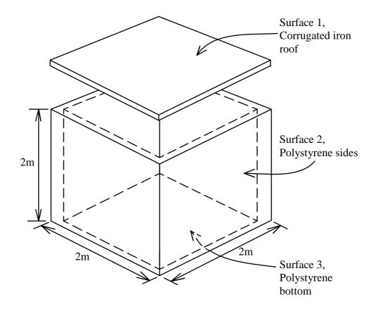
Figure C.1: Model for basis of radiation heat transfer calculation
