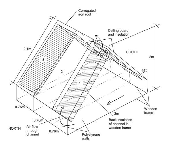
Figure 4.1: Proposed test-rig showing three separate compartments
