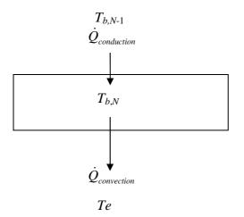
Figure C.6: Wall outer boundary control volume
