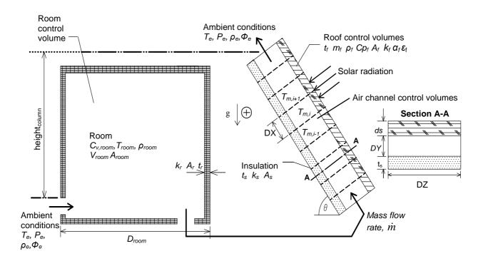
Figure 5.6: Most important parameters of summer analytical model
