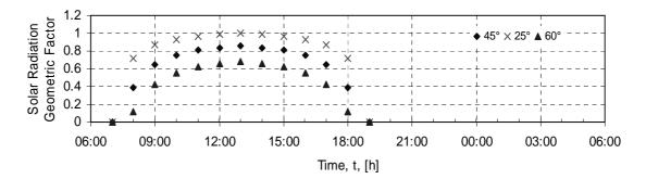
Figure B.8: Solar Radiation Geometric factor  $\zeta_s$  for summer
