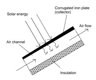
Figure 2.2: Sketch of proposed chimney design
