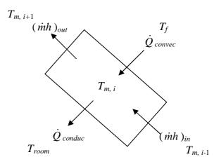
Figure 5.3: Sketch of air channel control volume
