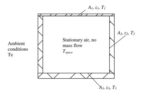
Figure C.2: Cross section of box for radiation effect calculations
