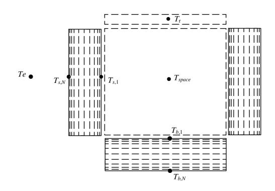
Figure C.4: Thermal model for polystyrene box
