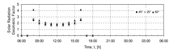
Figure B.3: Solar Radiation Geometric factor  $\zeta_w$  for winter
