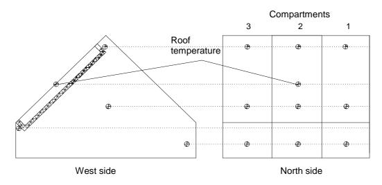
Figure 4.6: Placement of temperature sensors in the test-rig
