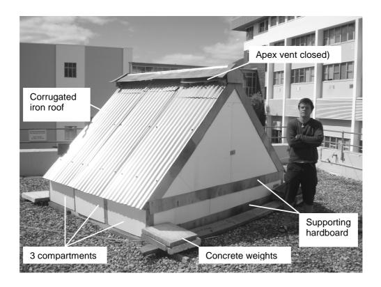
Figure 4.3: Test-rig built on site
