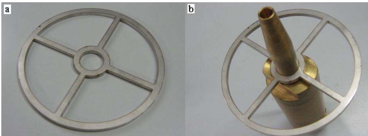
Figure 2.11: a) Stainless steel locator
