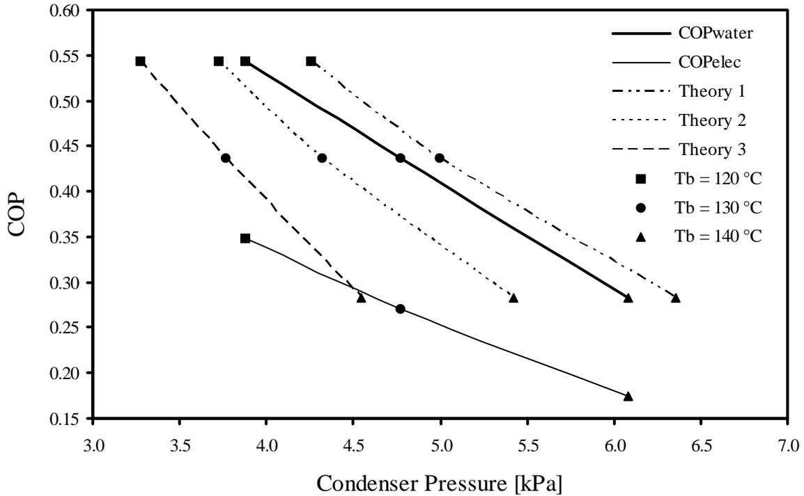
Figure 5.12: Water and electric COP compared to three theoretical models.  $T_e = 10\text{ }^\circ\text{C}$ ,  $A_R = 81$ ,  $NXP = 26\text{ mm}$  (Eames et al., 1995b)
