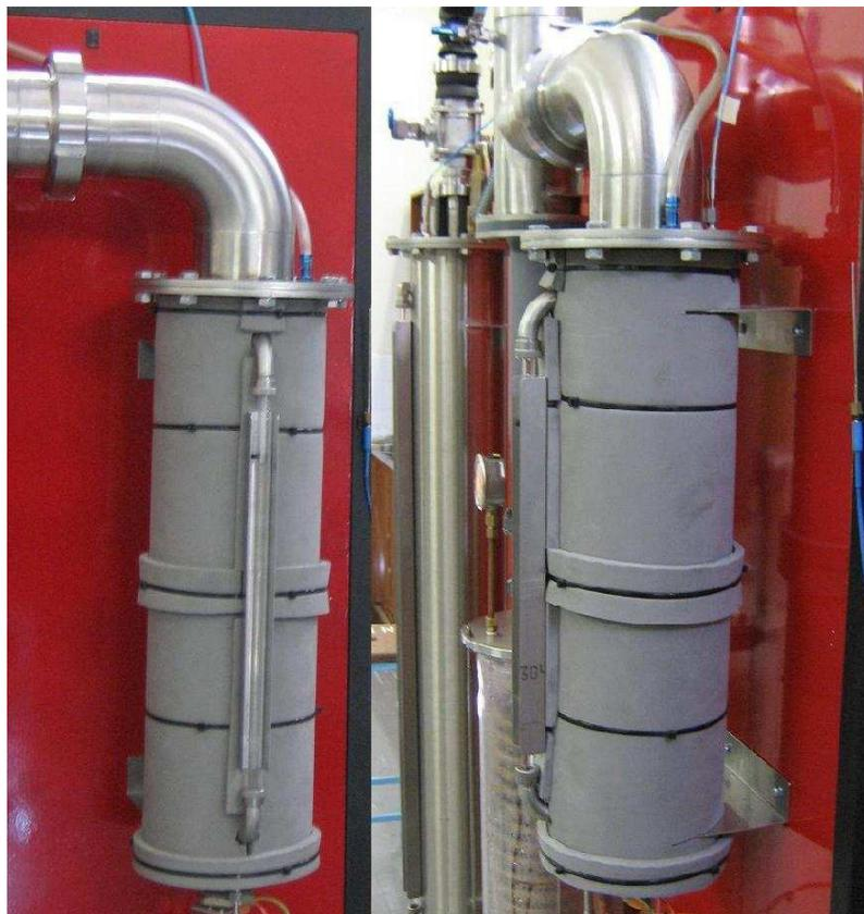
Figure 2.7: Partly insulated evaporator
