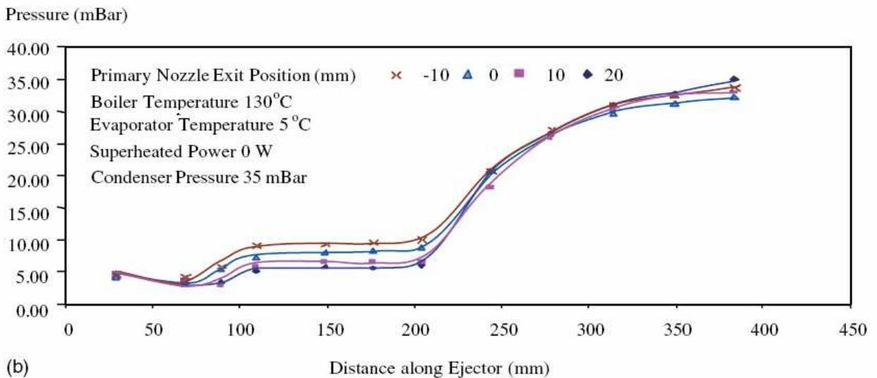
Figure 4.13: Steam ejector with varying primary nozzle exit position
