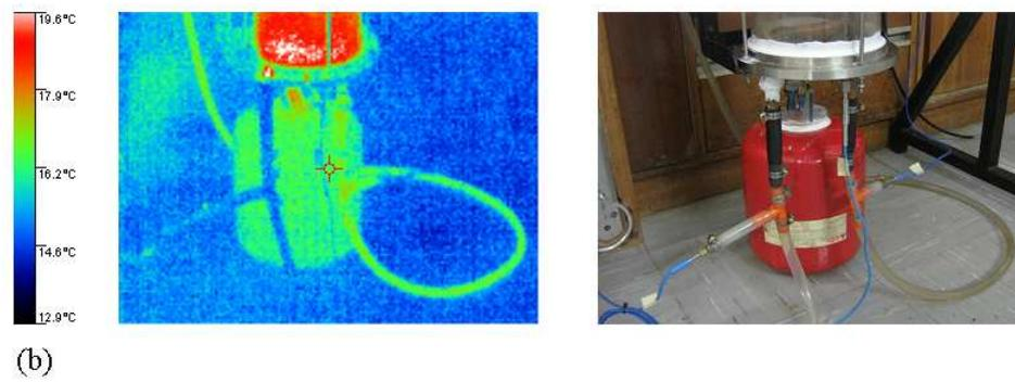
Figure B.3: IR and normal images of the condenser
