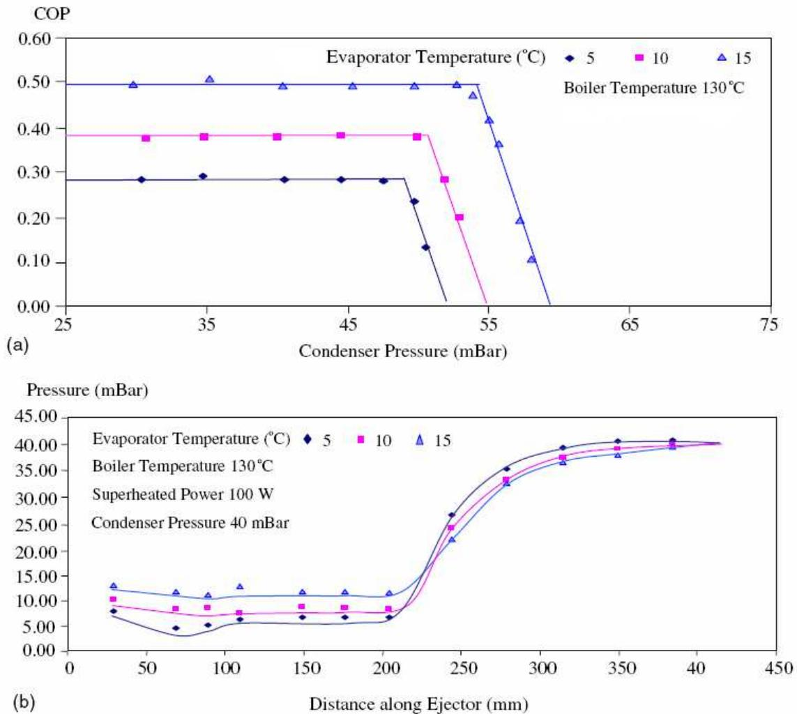
Figure 4.8: Steam jet ejector at different evaporator temperatures
