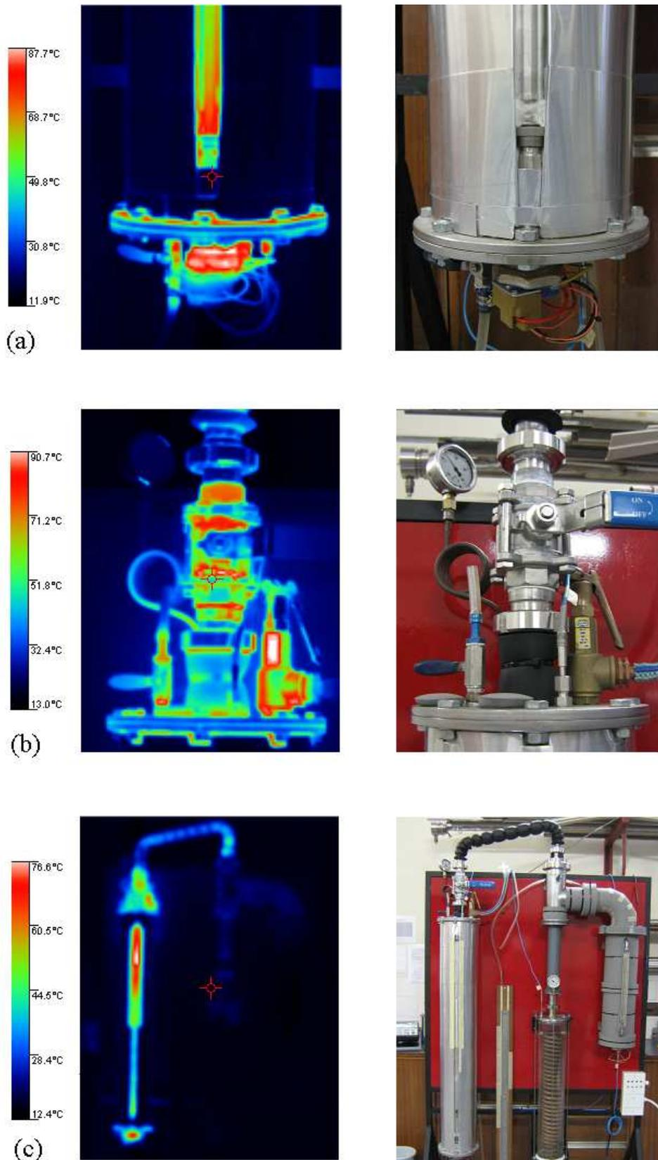
Figure 5.17: Infrared images pertaining to boiler heat losses
