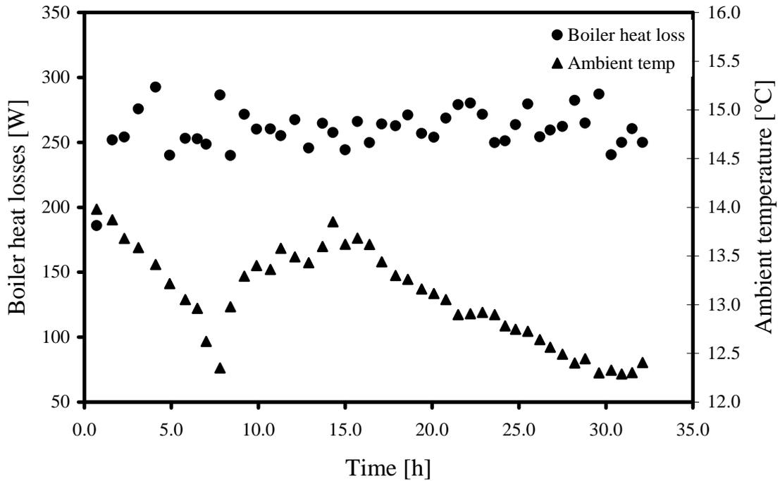
Figure 5.19: Boiler heat losses and ambient temperatures during a boiler insulation test at  $T_b = 100\text{ }^\circ\text{C}$
