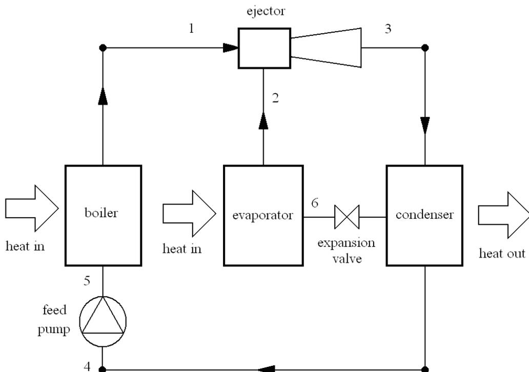
Figure 2.1: Ejector cycle (Chunnanond and Aphornratana, 2004b)
