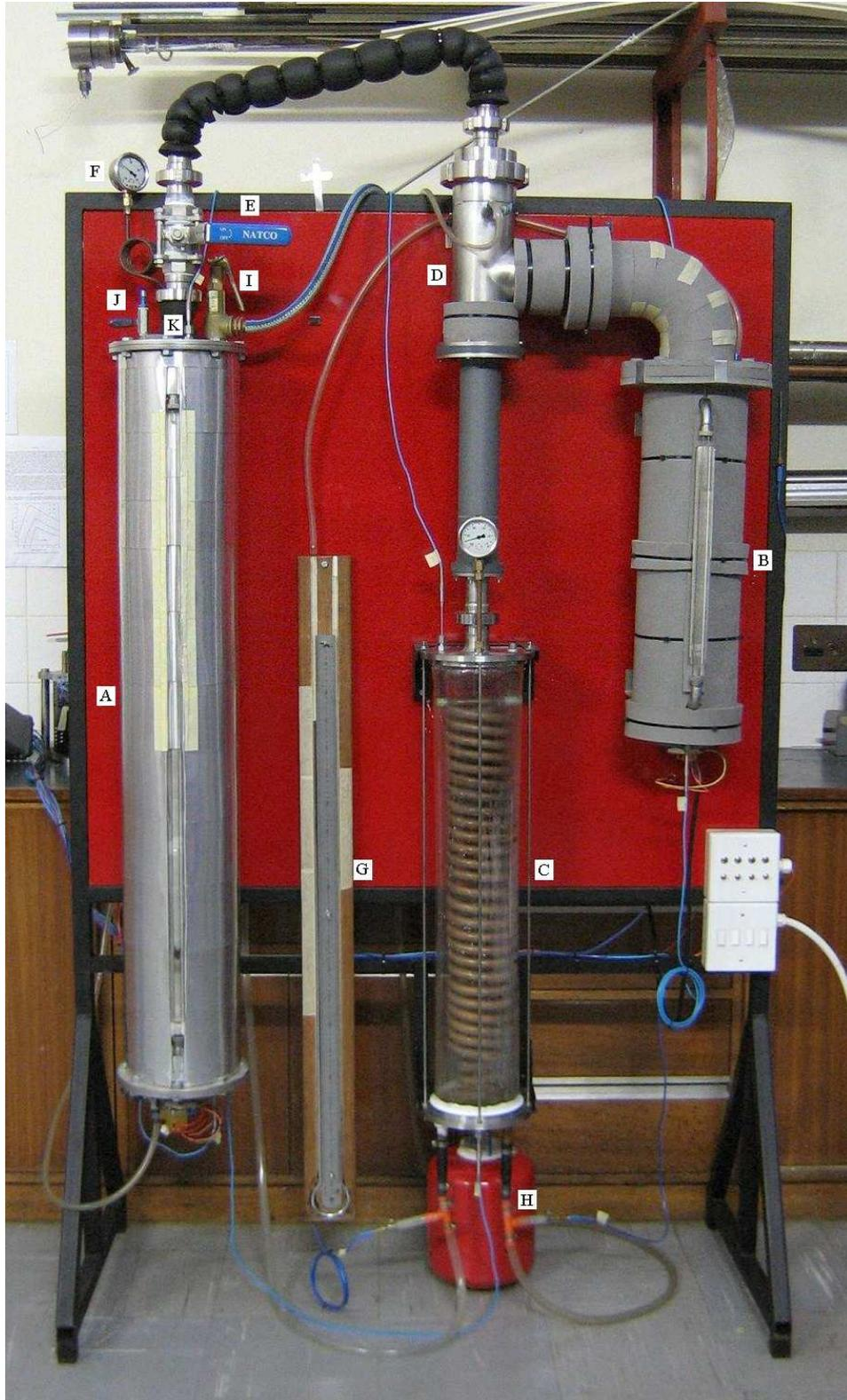
Figure 2.4: The ejector experimental setup
