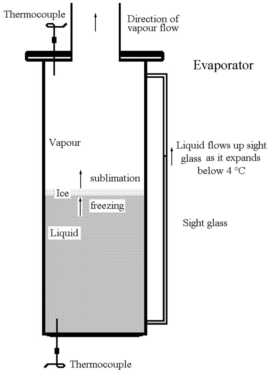
Figure 5.10: The evaporator during subzero vapour temperatures
