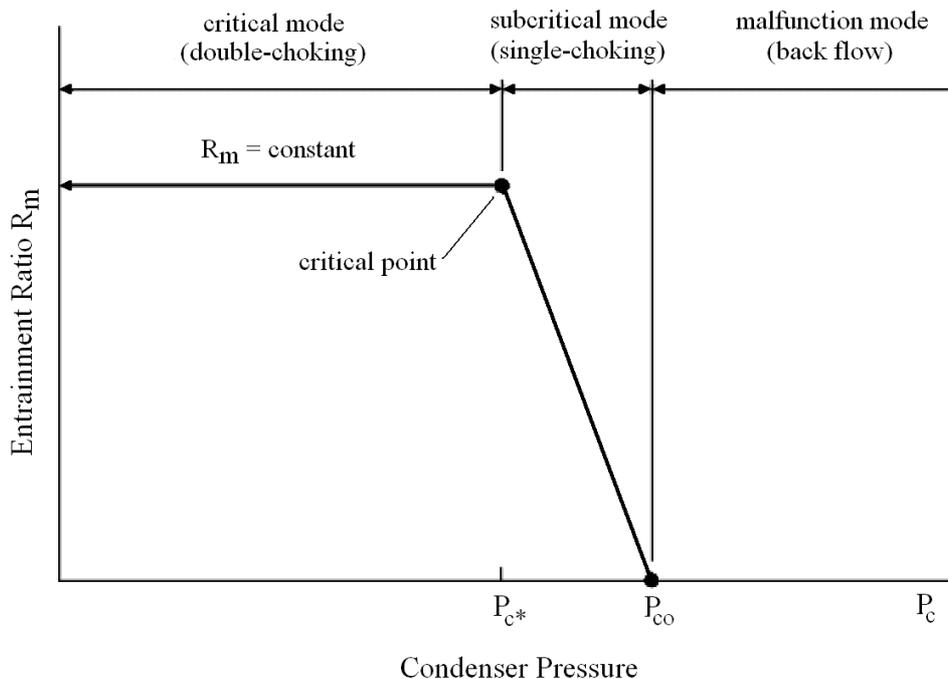
Figure 4.1: Operational modes of an ejector (Huang and Chang, 1999)
