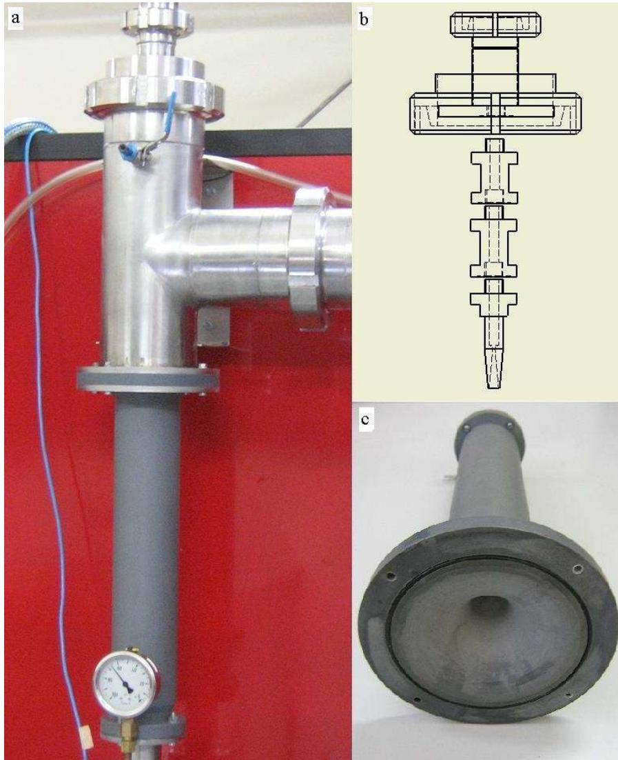
Figure 2.9: The ejector assembly
