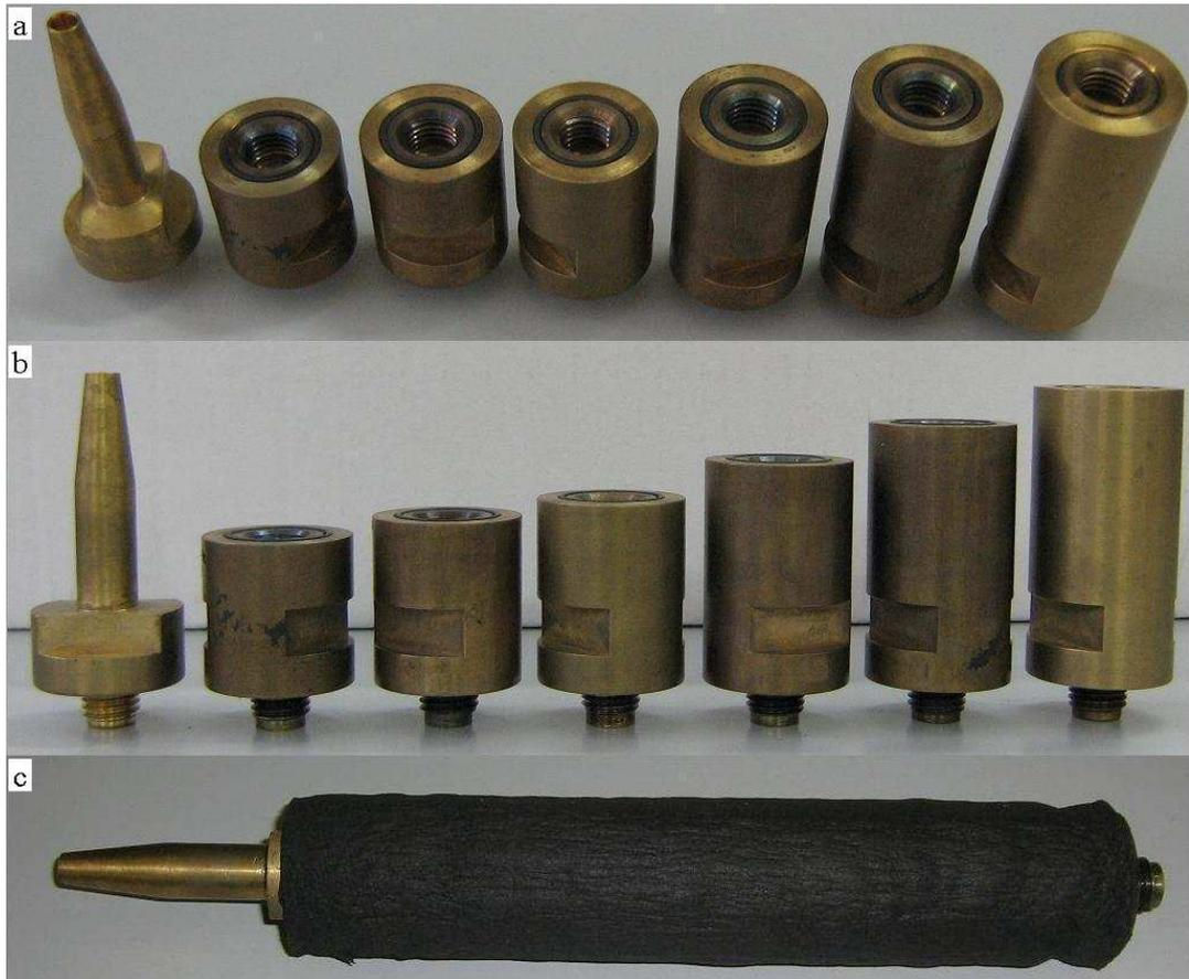
Figure 2.10: a,b) The nozzle and spacer
