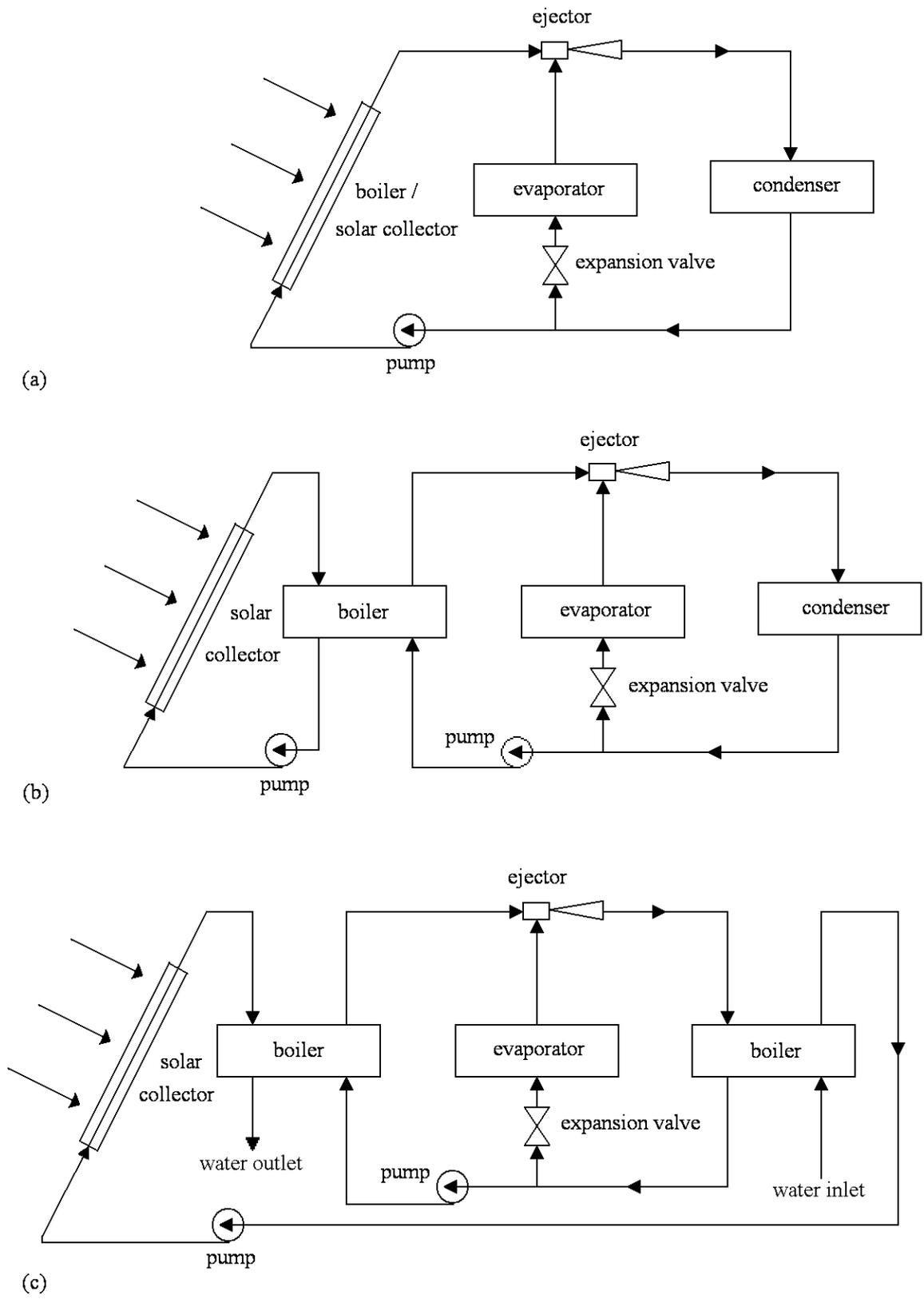
Figure 6.8: Solar powered ejector configurations (Sun and Eames, 1995)
