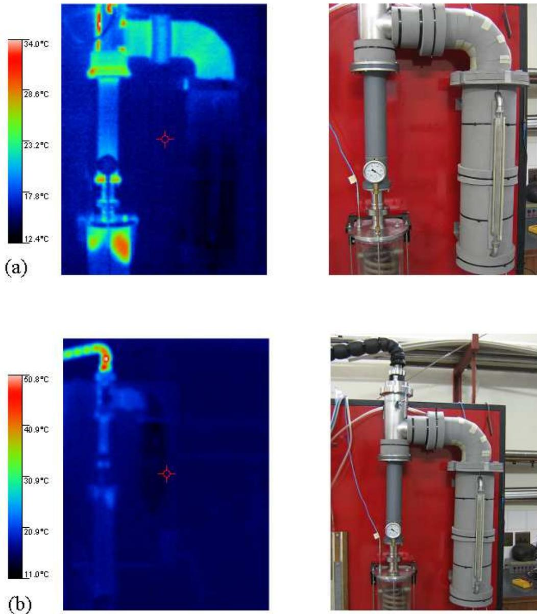
Figure B.5: IR and normal images of the evaporator
