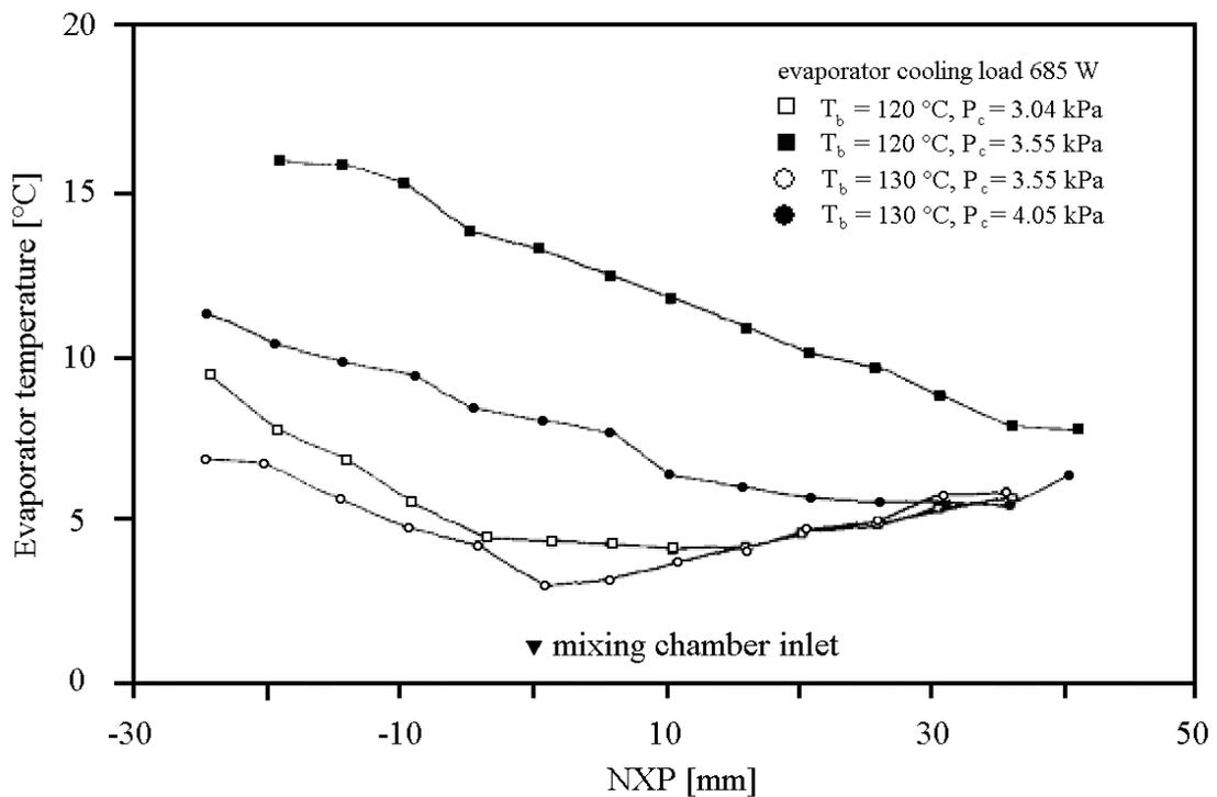
Figure 4.10: Measured evaporator temperature versus primary nozzle exit position (NXP), boiler temperature and condenser pressure (Aphornratana and Eames, 1997)
