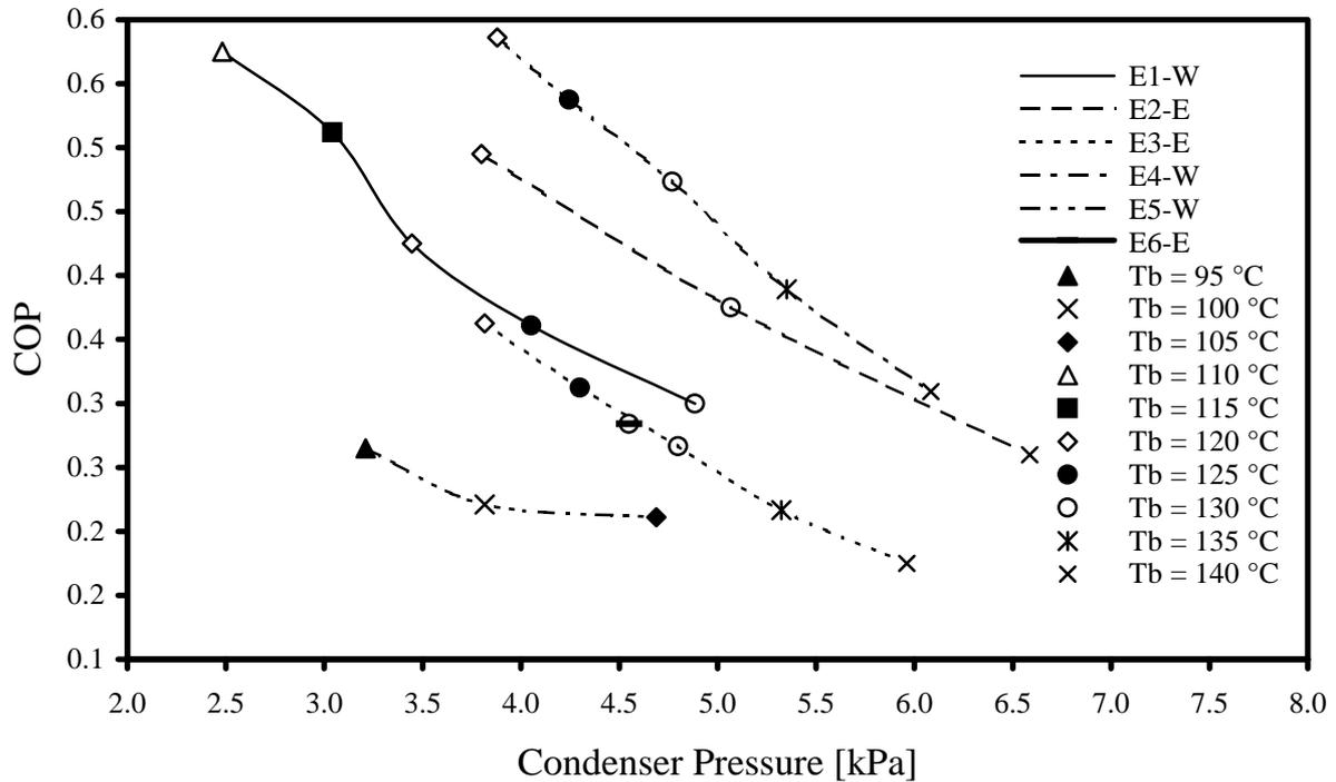
Figure 5.14: Comparison of different published data for  $T_b = 95\text{ }^\circ\text{C}$  to  $140\text{ }^\circ\text{C}$  and  $T_c = 10\text{ }^\circ\text{C}$
