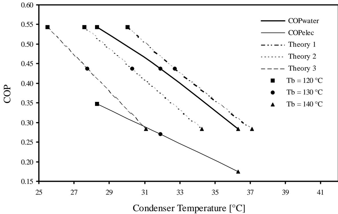
Figure B.6: Water and electric COP compared to three theoretical models.  $T_e = 10^\circ\text{C}$ ,  $A_R = 81$ ,  $NXP = 26\text{ mm}$  (Eames et al., 1995)
