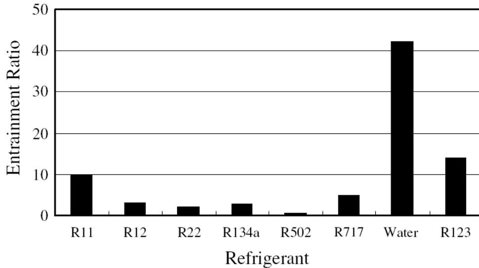
Figure 6.5: Entrainment ratio for vapour-liquid ejector for different working fluids (Shen et al., 2005)
