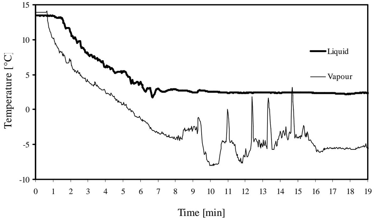
Figure 5.8: Evaporator temperatures versus time
