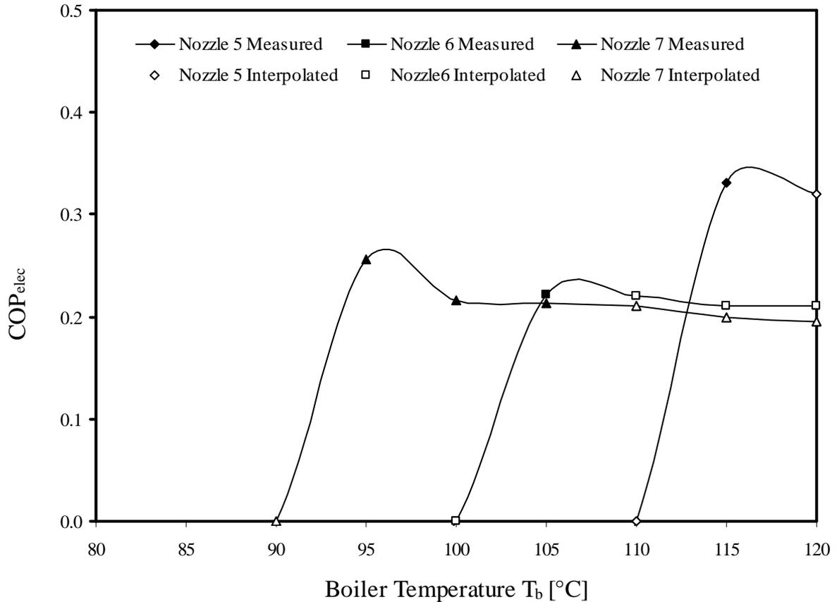
Figure 5.4: COP versus boiler temperature for different primary nozzles ( $P_c \geq 2.34$  kPa,  $T_c \geq 20^\circ\text{C}$ ,  $T_e = 10^\circ\text{C}$ ,  $NXP = -5$  mm)
