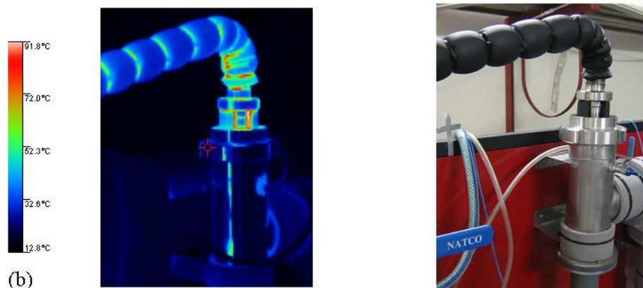
Figure B.4: IR and normal images of the steam pipe
