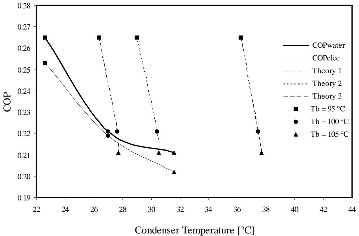
Figure B.7: Electric and water COP compared to three theoretical models.  $T_b = 95\text{ }^\circ\text{C}$  to  $105\text{ }^\circ\text{C}$ ,  $T_c = 10\text{ }^\circ\text{C}$ ,  $A_R = 26.5$
