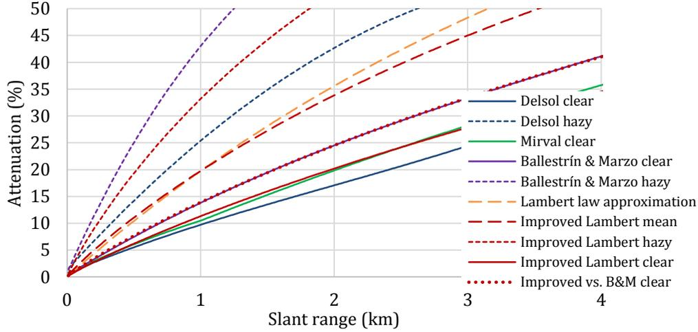
**Figure 5.13: Attenuation loss models**
