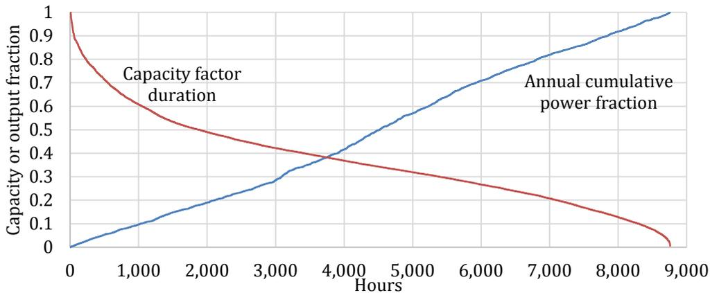
**Figure 6.12: Combined system wind power performance indicators; capacity factor duration curve (as a fraction by ranked hour) and annual cumulative power output (as a fraction by year hour)**
