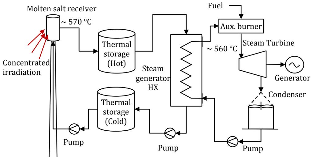
**Figure 5.4: Schematic layout of the central receiver CSP plant for the model**
