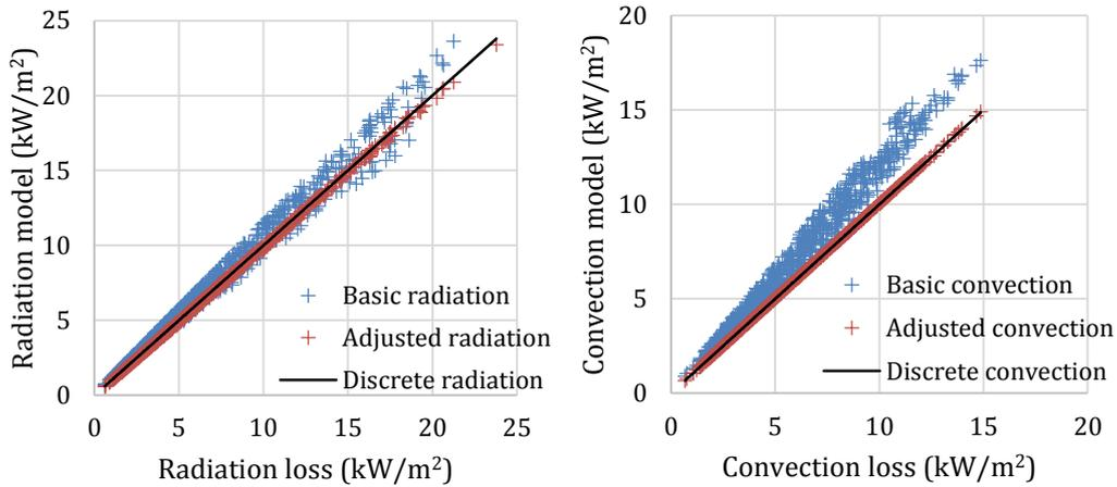
**Figure 5.16: Receiver model correlation for radiation (left) and convection (right)**
