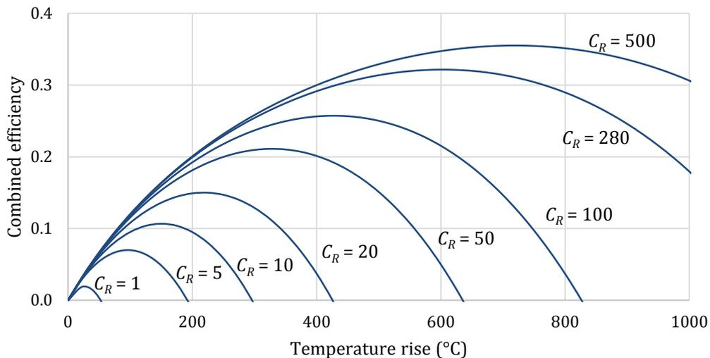
**Figure 2.7: Basic combined receiver and heat engine efficiency**
