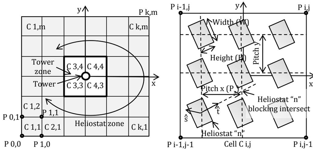
**Figure 5.6: Plan view of heliostat field zones and cells (left) and one heliostat cell (right)**
