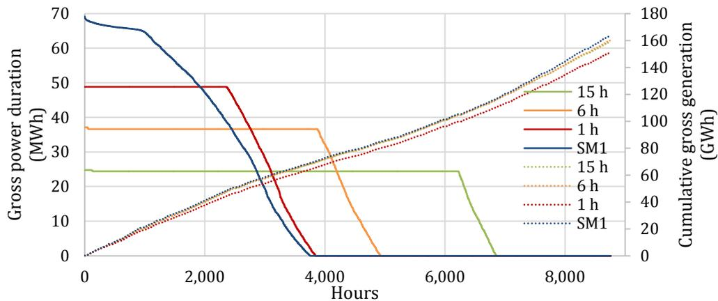
**Figure 5.26: Duration and cumulative generation of gross power curves for storage ratings of 15 hours, 6 hours, 1 hour and a case where the solar multiple is 1 and thermal energy passes through a 1 hour storage system**
