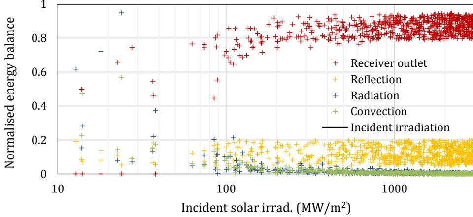
**Figure 5.20: Receiver energy balance model disaggregation normalized with logarithmic independent axis**
