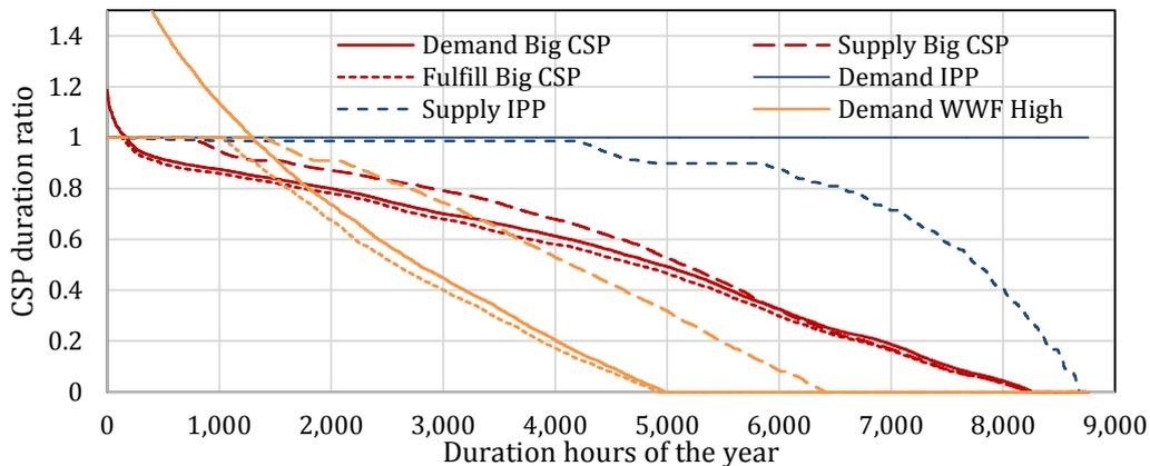
**Figure 8.12: CSP residual duration curves**
