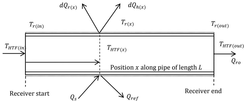
**Figure 5.15: Generic representation for the receiver energy balance**
