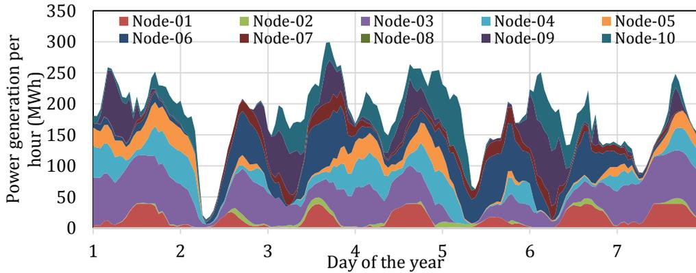
**Figure 6.11: First week of January at all wind nodes in the system and 500MW of capacity in this example**
