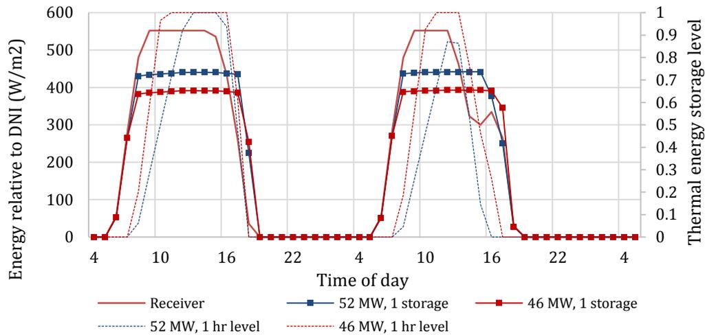
**Figure 5.24: Impact of solar multiple and storage capacity**
