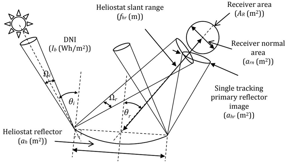
**Figure 5.5: General heliostat-receiver optics illustrated in 2D. Two edge incidence and reflected cones are shown.**
