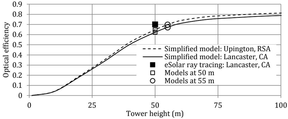
**Figure 5.8: Comparison of cosine, shading and blocking vs. tower height (defined as midpoint of receiver above heliostat field)**
