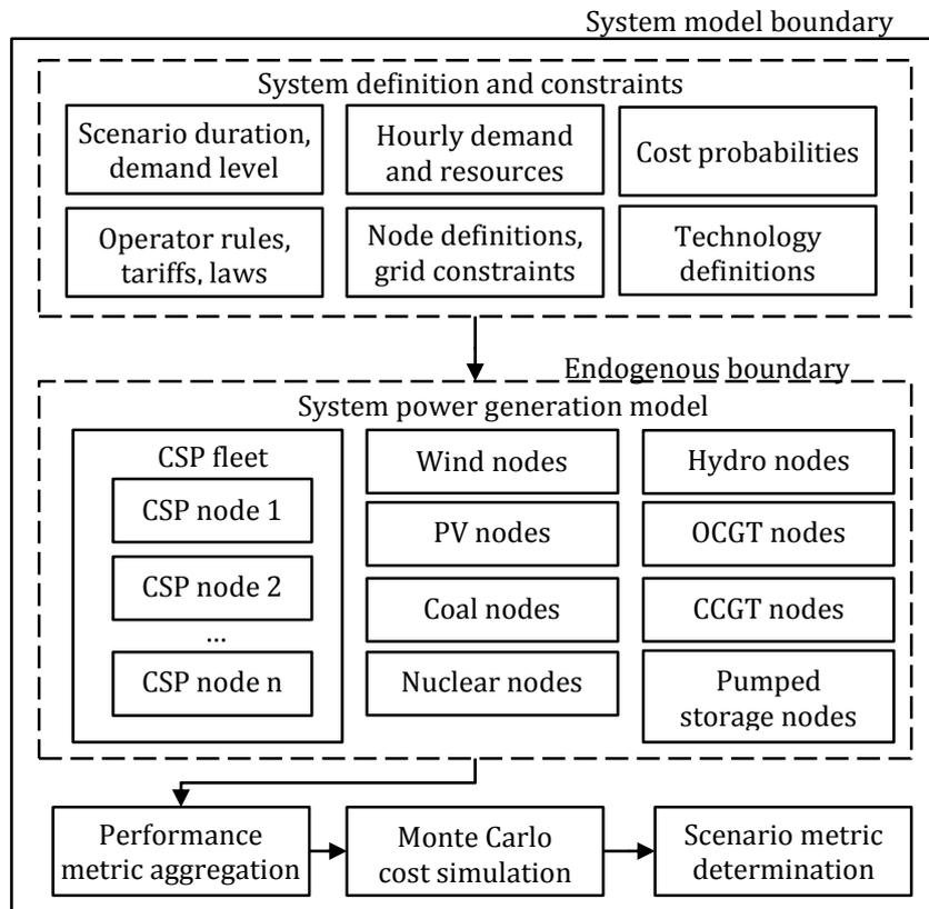
**Figure 6.1: Overall scenario system model structure and boundaries**
