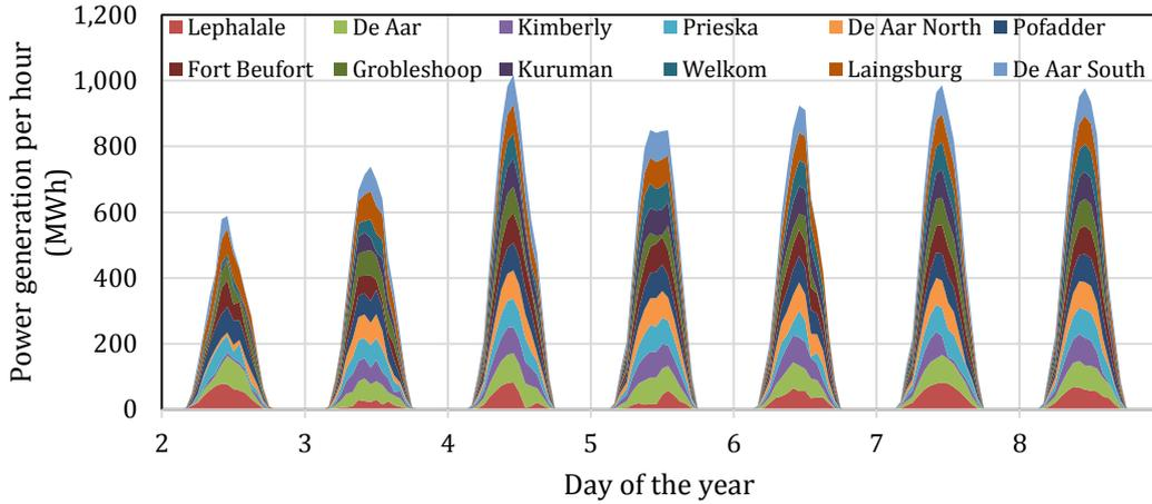
**Figure 6.8: Behavior of PV plant output for the twelve model nodes containing 100MW each – seven days of January**
