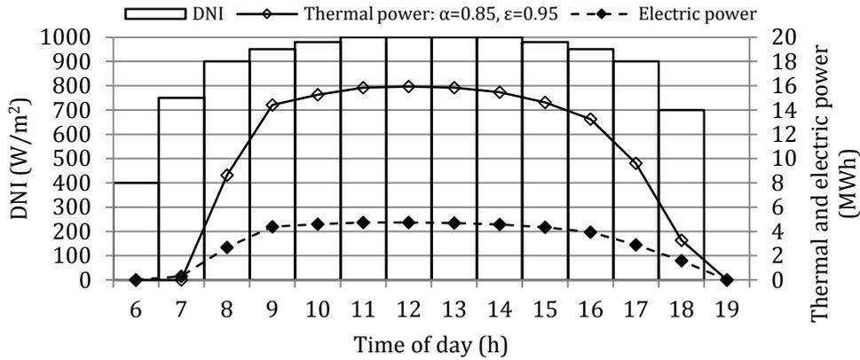
**Figure 5.27: Simplified model of thermal and electric power**
