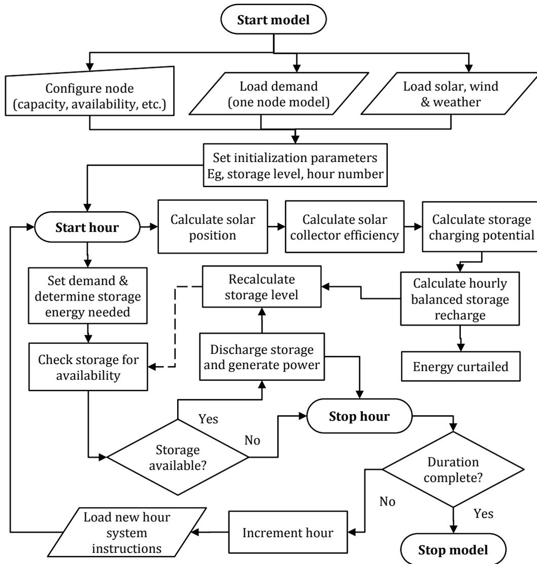
**Figure 5.3: Overall CSP model structure flow diagram**
