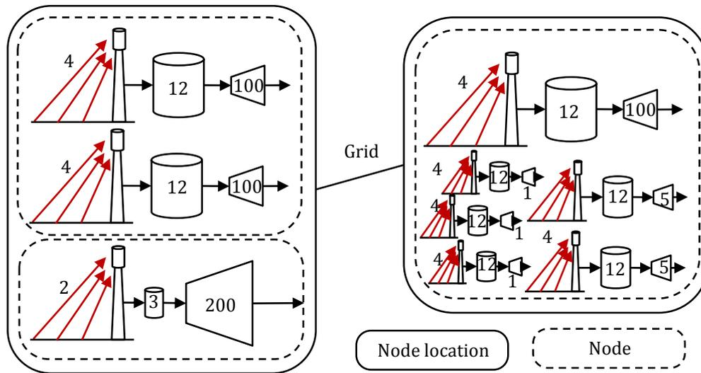
**Figure 5.2: Illustrative definition of nodes for proportioned capacities of CSP**
