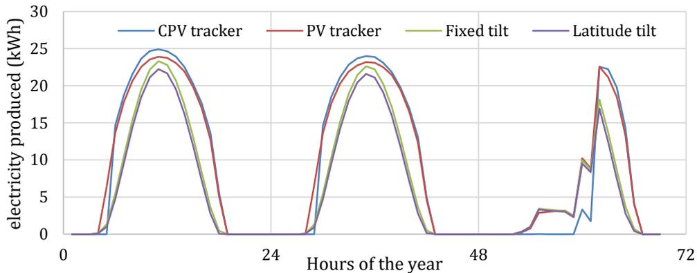
**Figure 6.7: Model of four PV configurations over a three day period in early summer near Stellenbosch University**
