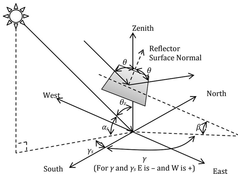
**Figure 2.3: Solar and heliostat angles for the CSP model**
