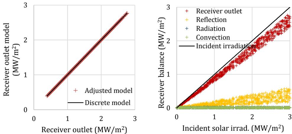
**Figure 5.19: Receiver model correlation for outlet energy (left) and disaggregation by incident irradiation (right)**
