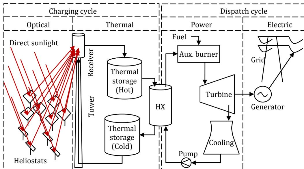
**Figure 2.2: Schematic layout of a central receiver CSP plant with storage**
