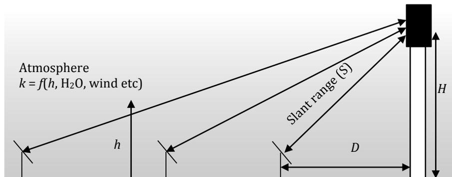
**Figure 5.12: Definition of slant range for atmospheric attenuation**
