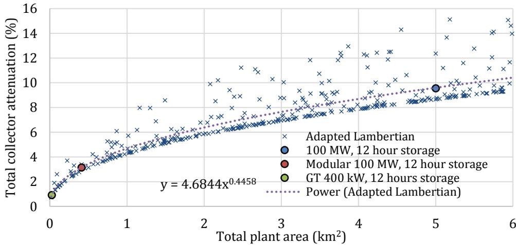
**Figure 5.14: Central receiver collector performance loss by attenuation**
