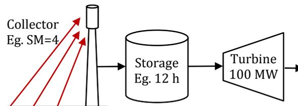
**Figure 5.1: Illustrative proportions of a CSP plant with a solar multiple (SM) of 4, 12 storage hours and a 100 MW turbine**
