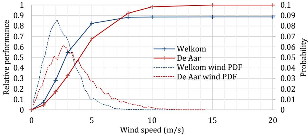
**Figure 5.11: Cumulative annual performance impact as a function of wind cutoff speed. Sites indicated use zero cutoff performance of best site as ratio denominator. Wind probability distribution is indicated by respective dotted lines.**
