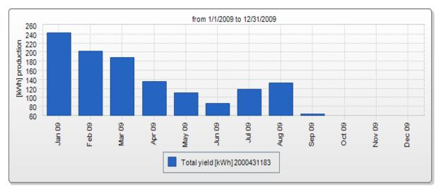
Figure 4.4: Energy yield for the 1.7 kW PV roof tile system at Lynedoch's guesthouse for the period 1/1/2009-31/09/2009
