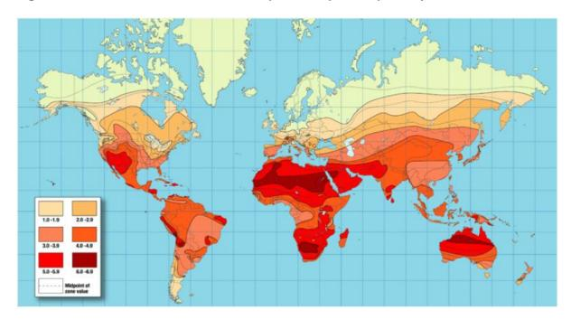
Figure 2.6: World solar insolation map – kWh per  $m^2$  per day
