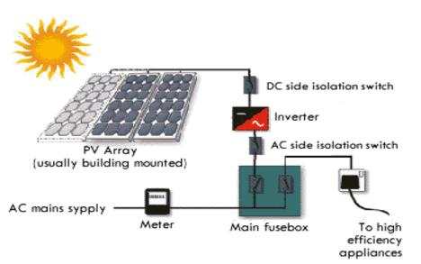
Figure 4.7: A diagram of a typical grid-connected PV system
