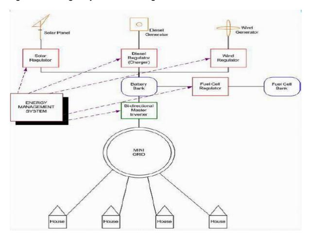
Figure 4.9: Mini-grid system connecting a number of users
