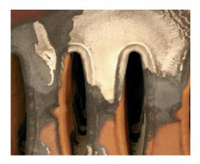
Figure 1.1: Corrosion on entrance to the ACC tubes Source: Dooley, Aspden, Howell & Du Preez, 2009.
