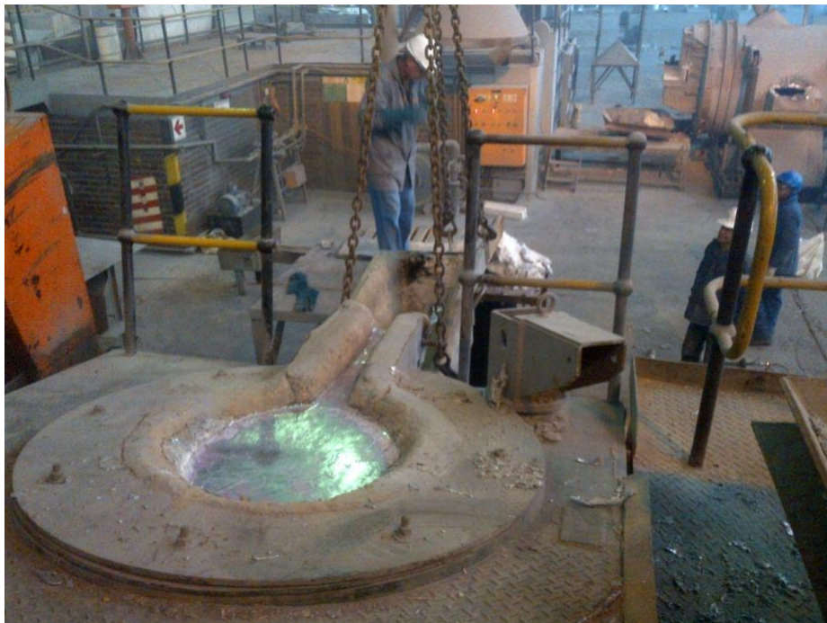
Figure 46 - Casting of AlSi12 into test section
