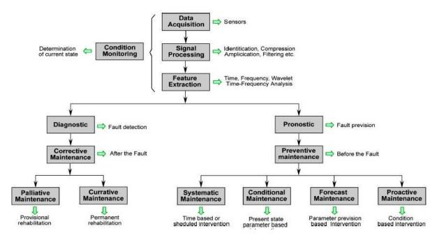
Figure 28: A breakdown of the condition based maintenance in wind turbines
