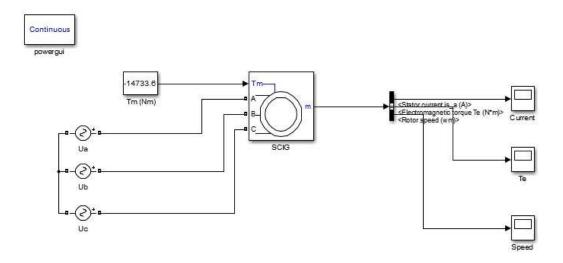
Figure 42: The complete SCIG Simulink model
