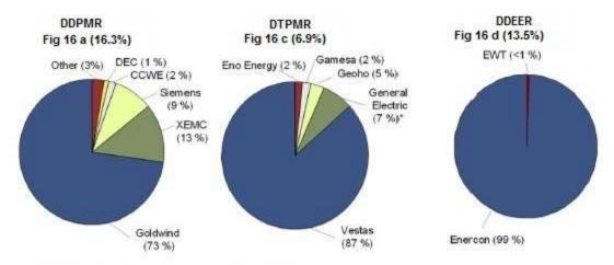
DDPMR - Direct Drive Permanent Magnet Rotor DTPMR - Drivetrain Permanent Magnet Rotor DDEER - Direct Drive Externally Excited Rotor
