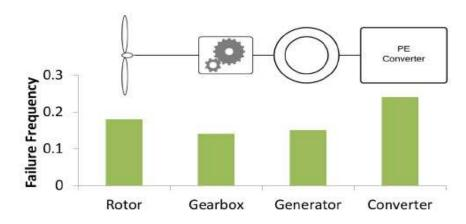
Figure 21: Drivetrain sub-assembly failure frequency
