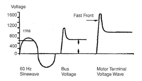
Figure 26: Voltage spikes generated by PWM circuits
