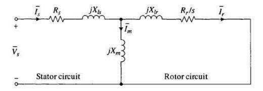
Figure 33: SCIG steady-state equivalent circuit
