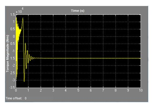
Figure 49: SCIG electromagnetic torque output
