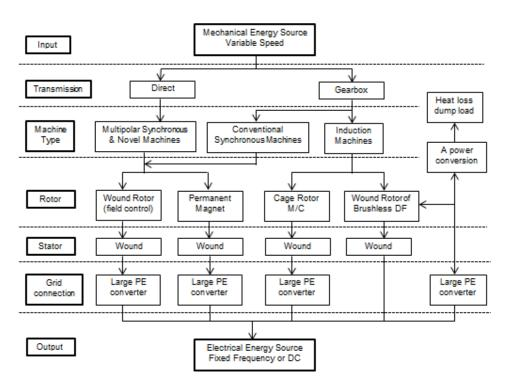
Figure 12: Road map: Power electronics converters for energy conversion in wind energy technologies
