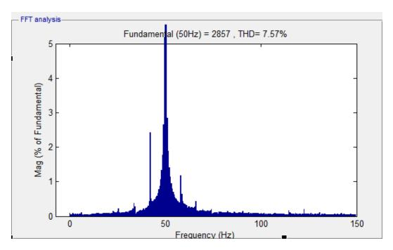
Figure 48: FFT analysis of stator phase current with 15% degradation
