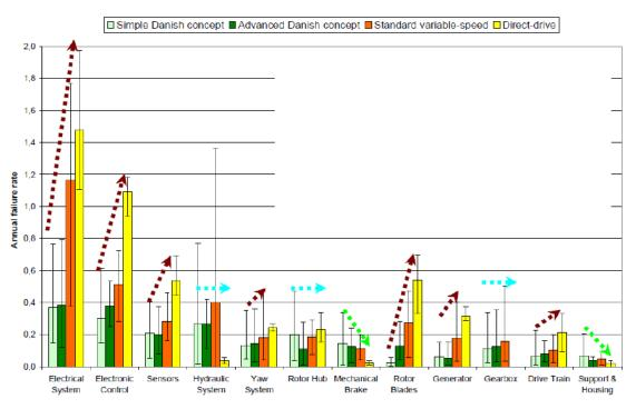
Figure 19: Different wind technology topologies and related failure
