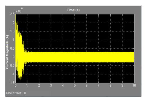
Figure 46: Stator phase current with 15% degradation
