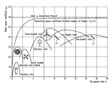
Figure 10: Power coefficients of different wind turbine designs
