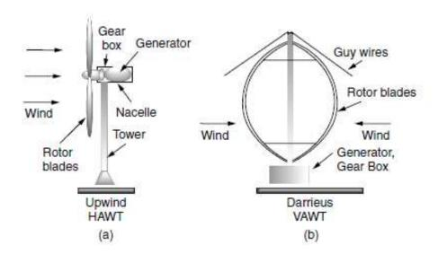
Figure 9: Wind turbine rotor designs
