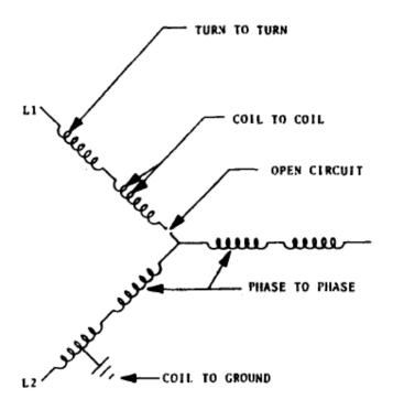
Figure 25: Stator winding failure modes
