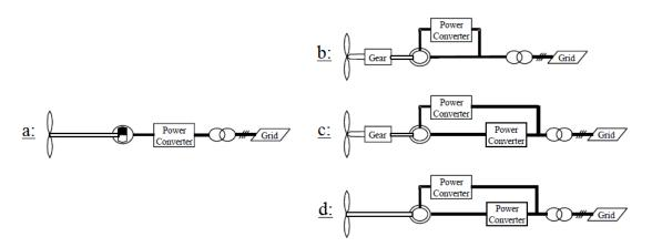
Figure 16: Variable speed wind turbines using synchronous generator concepts
