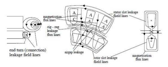
Figure 35: Different leakage flux flow
