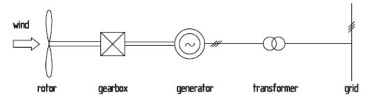
Figure 11: Electrical power conversion in WECs
