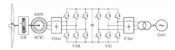
Figure 31: SCIG variable speed wind turbine configuration
