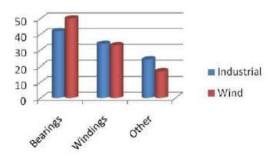
Figure 24: Electrical machine faults in wind turbines and industrial applications
