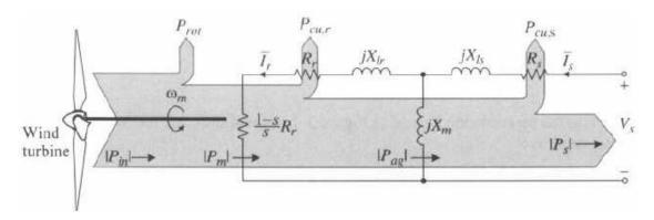
Figure 34: Induction generator power flow and machine losses
