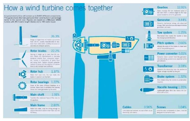
Figure 18: Cost contribution of main components and systems of a 5 MW wind turbine
