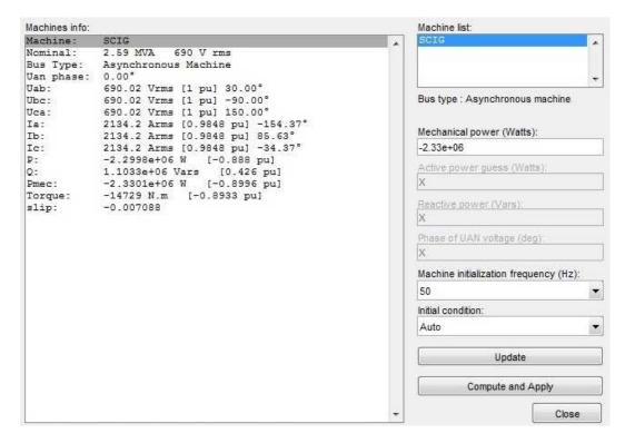
Figure 43: SCIG machine initialization calculations
