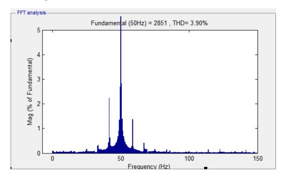
Figure 47: FFT analysis of stator phase current with zero degradation
