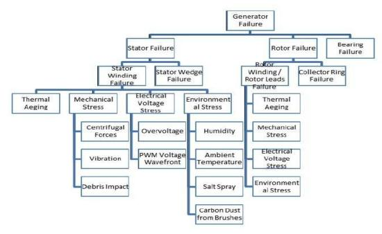
Figure 23: Typical wind turbine generator failure chart
