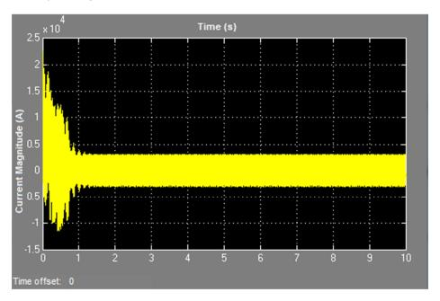
Figure 45: Stator phase current with zero degradation
