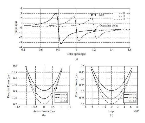
Figure 32: Steady state operating characteristics of a variable speed SCIG wind turbine
