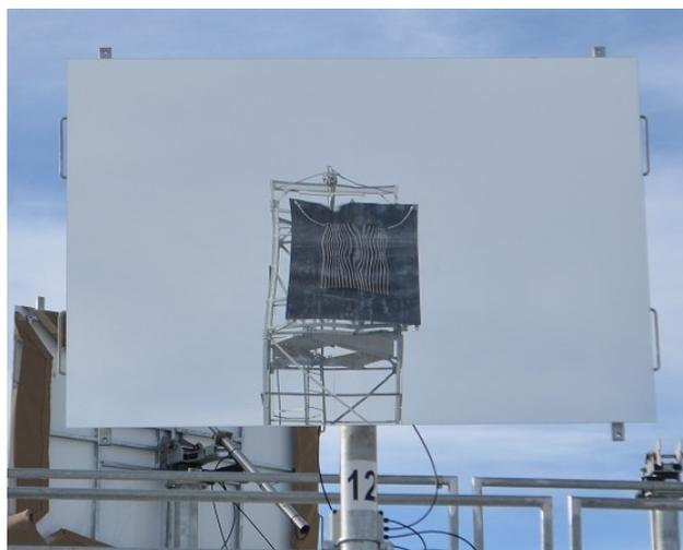
**Figure 7.2:** A Helio40 heliostat showing warping of the reflected image
