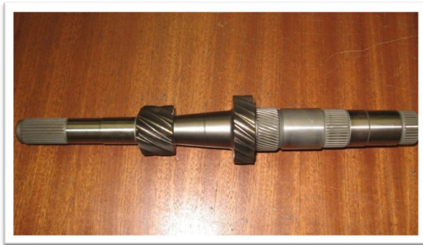
FIGURE 67 – SPLINED SHAFT FROM A POLO GEARBOX SUPPLIED BY VWSA
