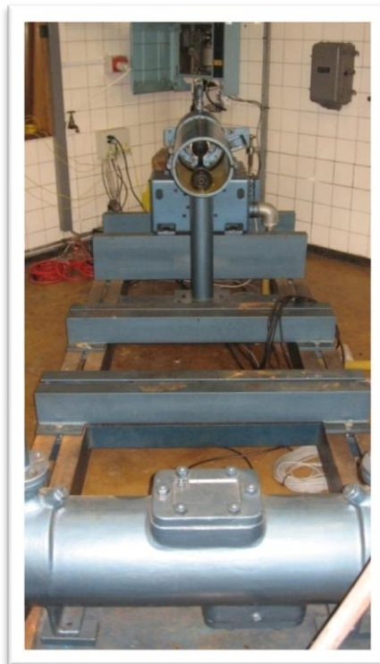
FIGURE 14 - STRIPPED DOWN TEST BED BEFORE ENGINE INSTALLATION
