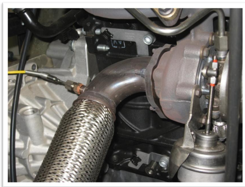
FIGURE 60 - EXHAUST THERMOCOUPLE INSTALLATION
