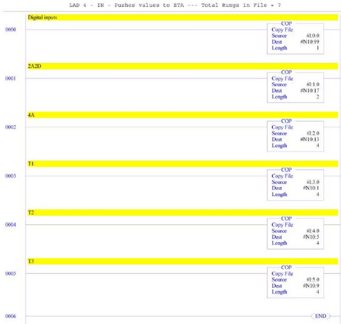
FIGURE 72 - PLC LADDER LOGIC PROGRAM (PALMER, 2008)
