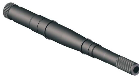
FIGURE 68 - SHAFT WITH GEARS GROUND OFF AND WITH BEARING LOCATORS MACHINED
