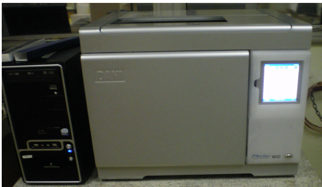
Figure 3-1 Dani Master GC instrument for glycerol and glyceride analyses.
