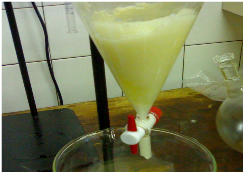
Figure 2-8 A transesterification reaction that formed soap due to excess of catalyst
