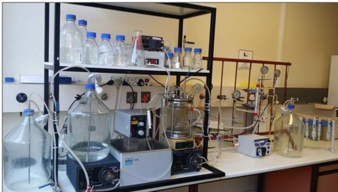
Figure 95: Experimental Set-up for MBR operation
