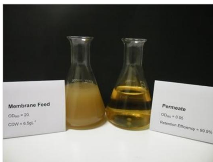
Figure 58: Optical examination of the retention efficiency of the MFU. Concentrated sample from culture mixture (left) and permeate (right)
