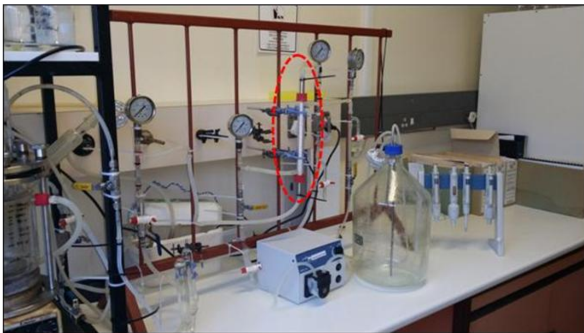
Figure 98: Single tubular membrane microfiltration unit (indicated by red ellipse), permeate reservoir, and backflush pump
