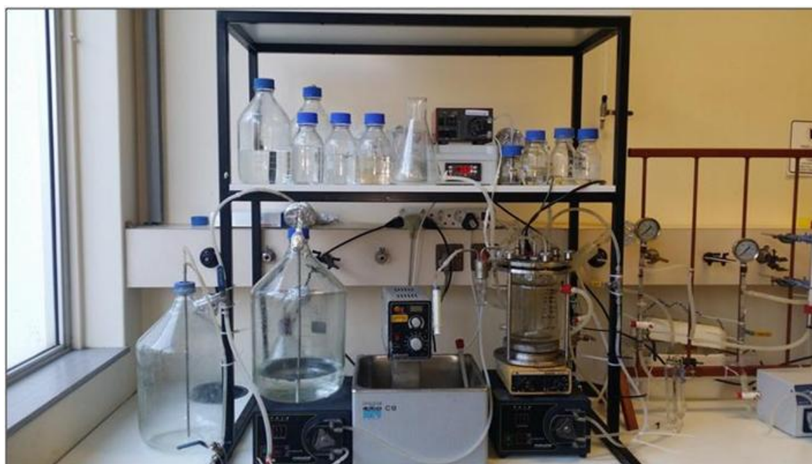
Figure 96: Custom built 1.5L fermenter, water bath, and fresh substrate reservoirs
