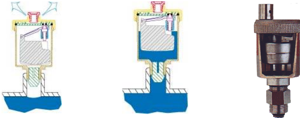
Figure 76: Automatic air eliminators (15,16)
