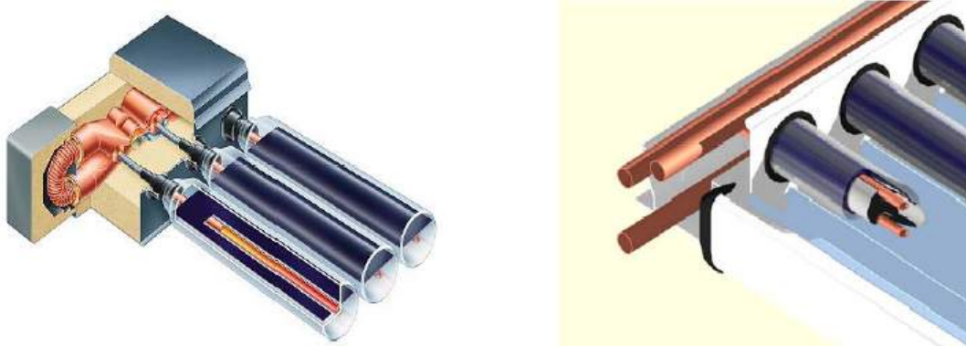
Figure 32: Evacuated tube collectors: Heatpipe, Vitosol 300 (left) and a direct coupled Sydney Collector (right)
