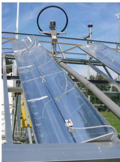
Figure 104: Testing of parabolic trough collectors at AEE INTEC in Austria.
