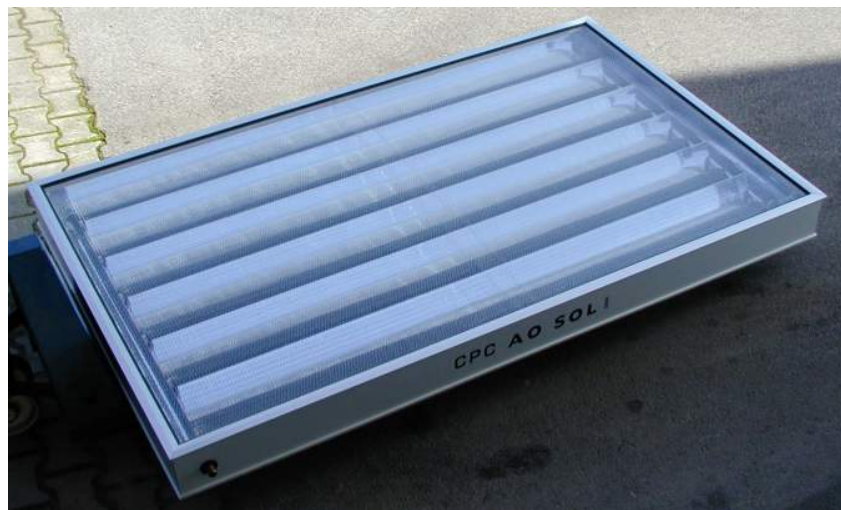
Figure 103: CPC collector : 1,12 – 1,7 x, acceptance angle: 37 – 56° (Source: Ao Sol Portugal)
