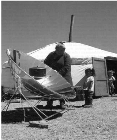
Figure 40: Concentrating solar cooker, south west of Ulan Bator, Mongolia
