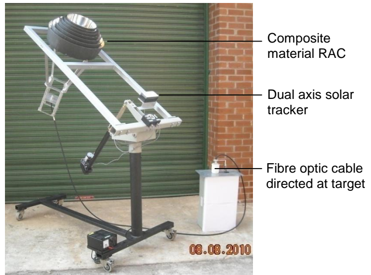
Figure 1. The Fibre Optic Concentrating Utilisation System developed for high temperature applications. Preliminary testing at the 20 mm diameter concentrator focal point achieved temperatures exceeding 1400^{\circ}\text{C} .
