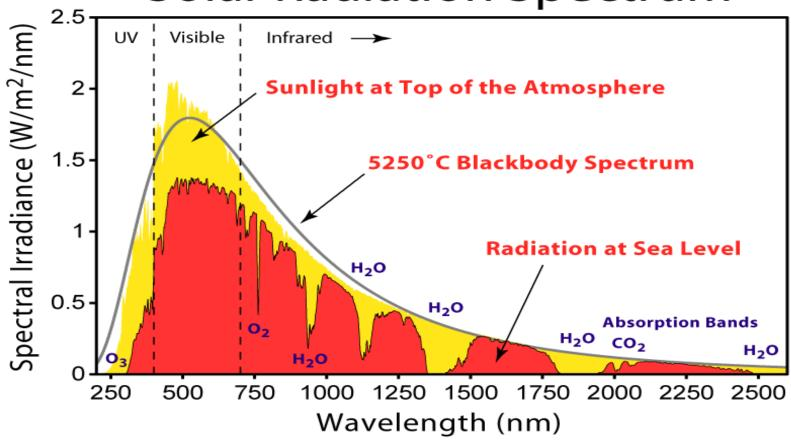
Solar radiation spectrum of at an average solar constant of I0=1353 kWh/m<sup>2</sup> Source: http://www.howtopowertheworld.com
