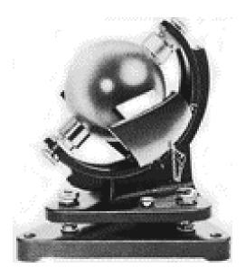
It consists of a solid glass sphere as a lens that produces an image of the sun on the opposite surface of the sphere. A strip of inflammable paper is mounted around the appropriate part of the sphere, and the solar image burns a mark on the paper whenever the beam radiation is above a critical level. If the sun is covered by clouds, the line on the paper is interrupted. The lengths of the burned portions of the paper gives and index of the duration of bright sunshine.
