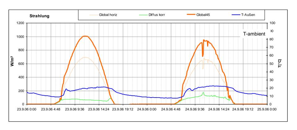
Global radiation on the horizontal and a 45° inclined surface for two clear days, latitude 47°.
