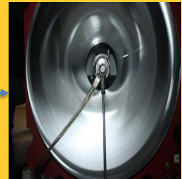
Reflector with Xe-Arc Lamp
