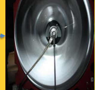
Reflector with Xe-Arc Lamp
