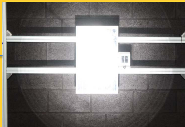
Target Area with Reference cell and C-Si Module
