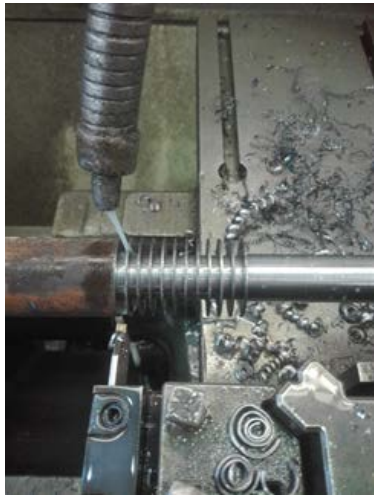
Figure 5: Machining of the fins
