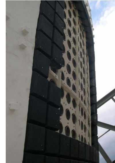
Fig 2: HiTRec II absorber modules assembled in a 3MW (thermal) receiver (Avila Marin, 2011)
