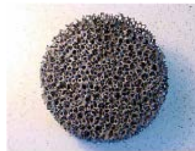
Fig 4: Open Cell Structure (Fend,2004)
