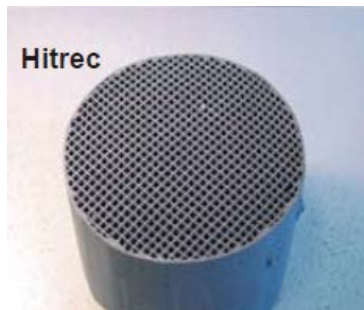
Fig 3: Monolith Honeycomb Structure (Fend,2004)
