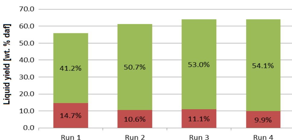
Figure 7. Overall pyrolytic water yield for the KIT 10 kg/h FP plant: Pyrolytic water (■ bottom); and Organic condensates (■ top)
