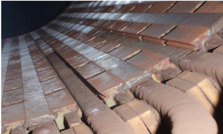
**Figure 27: Missing stator slot wedges**
