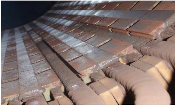
**Figure 27: Missing stator slot wedges**
